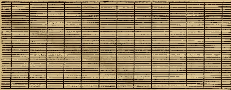
PLATE B. Horizontal divisions, 4 to the inch. Vertical divisions, 30 to the inch; each tenth horizontal and every twenty-fifth vertical division line heavier than the rest.
