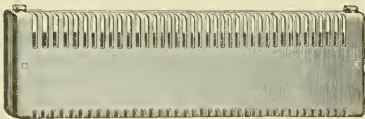
STYLE C HEATER UNDER CROSS SEATS—METROPOLITAN ELEVATED.
