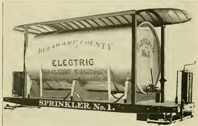
JACKSON & SHARP SPRINKLER.
