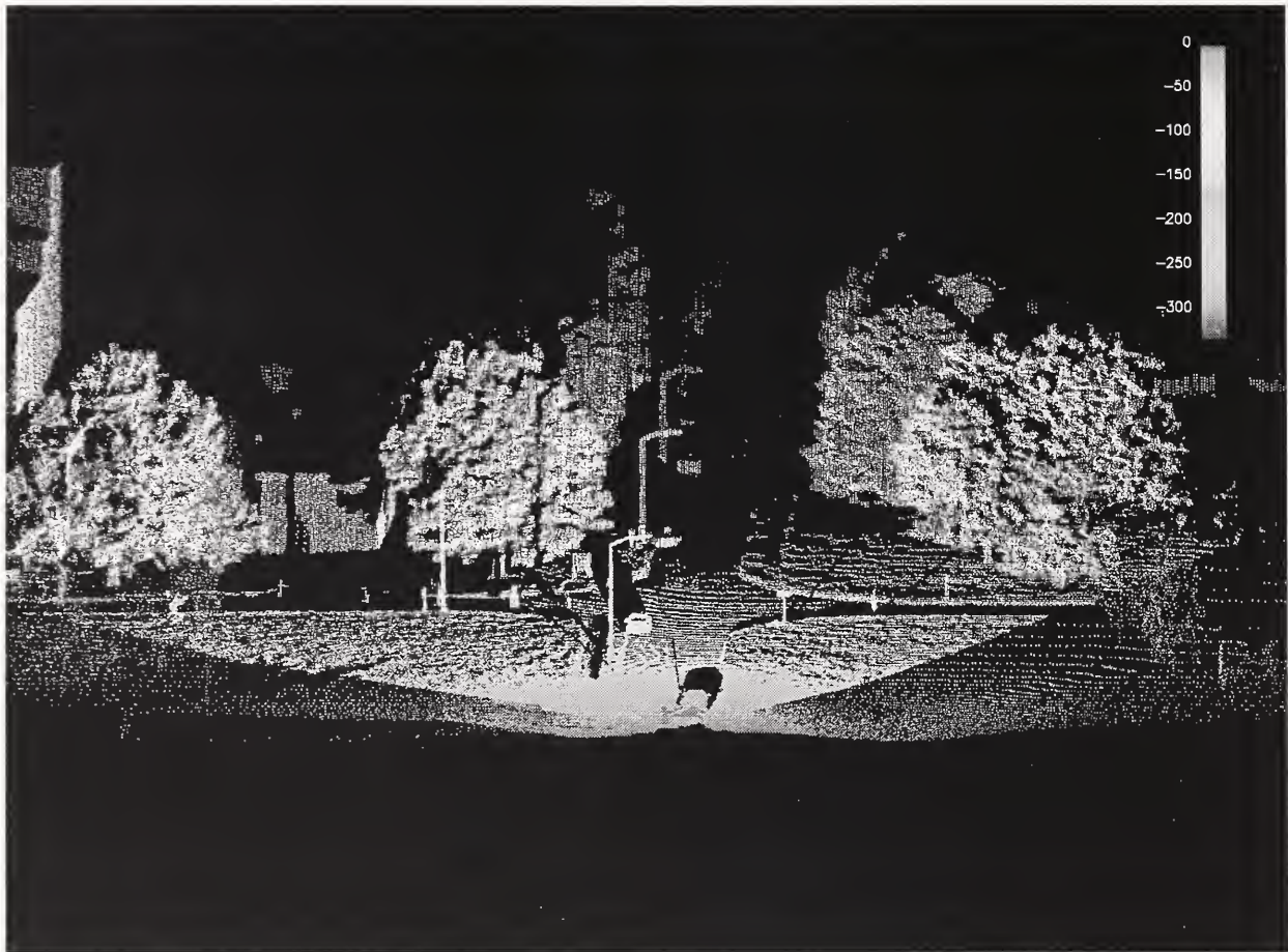
Figure 4-3 A LADAR point cloud taken from the same position as the photo in Figure 4-2. The image is color coded for distance. Red is zero. Green is about 175 m. See scale at top right. Note the four cars. The car at 150 m is clearly visible. Returns from the ground disappear at about 75 m.
