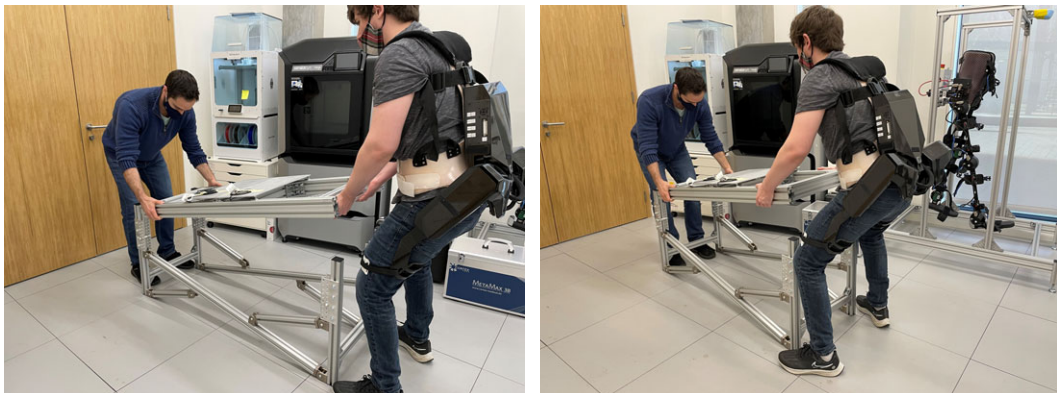
Figure 6. Snapshots of an example triadic collaboration work task involving two human agents and an exoskeleton. One human agent bears the brunt of the load, with the assistance of an exoskeleton providing ergonomic support. Meanwhile, the second human agent carries out the finer manipulation.
