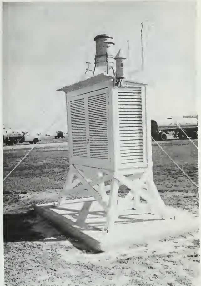
Figure 4-4.—Shelter used with AN/GM Q-14 ( ).
