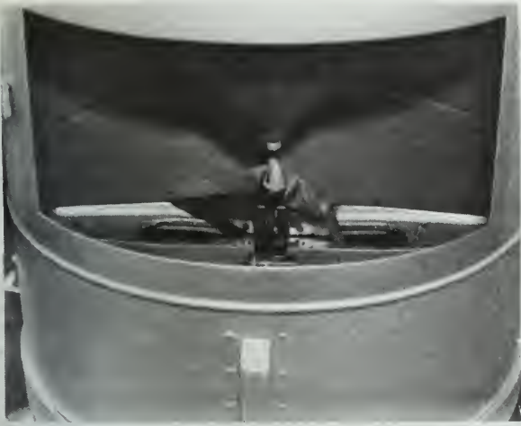
209.401 Figure 4-18. — Tipping bucket rain gage, with door open showing the two-compartment tipping bucket on its pivot.
