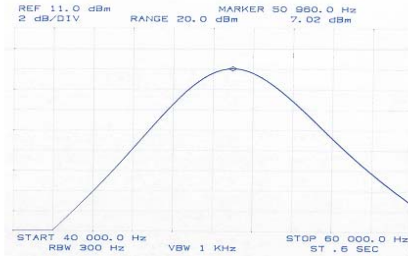
Figure 53. Actual Frequency Response: Center Frequency = 50.560 kHz, Q_p = 9.711
