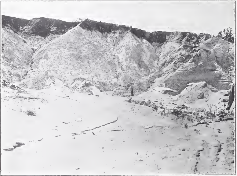
FIG. 5.—Clay pit in Wilcox formation near Holly Springs, Miss. To the right of view the sand rises almost to the surface. At the left of view the clay rises to the surface. This shows the irregular occurrence of the clay in this region. Dark overburden is loam.
