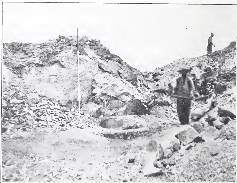
FIG. 16.—Mass of diaspore clay in flint clay deposit near Hofflin, Mo. The rod stands in front of a mass of diaspore clay. The man in foreground is standing on flint clay.
