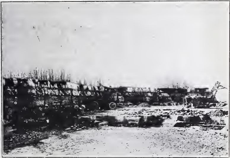
FIG. 1.—Behan's quarry, Manlius, Onondaga County, New York. The upper level of the quarry floor and the second heavy bed from the top of the quarry face were the productive cement layers.
