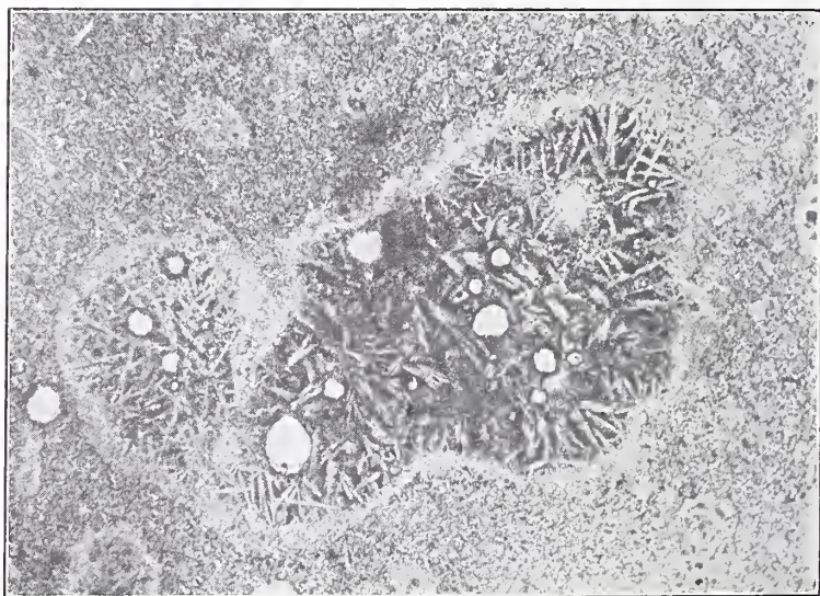
FIG. 4.—Photomicrograph of a thin section of the clinker from Burn No. 3. Mag. 50x.
