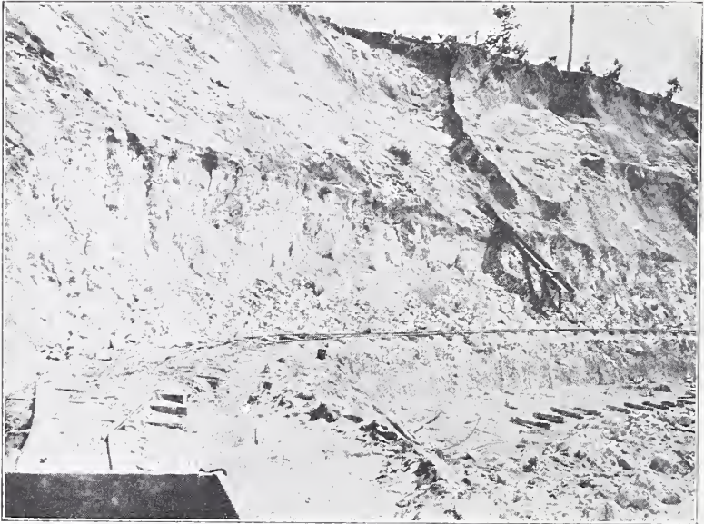
FIG. 3.—White clay overlying bauxite in Sweetwater mine, near Andersonville, Ga. Railroad tracks at upper limit of bauxite. White clay overlain by iron-stained sands.
