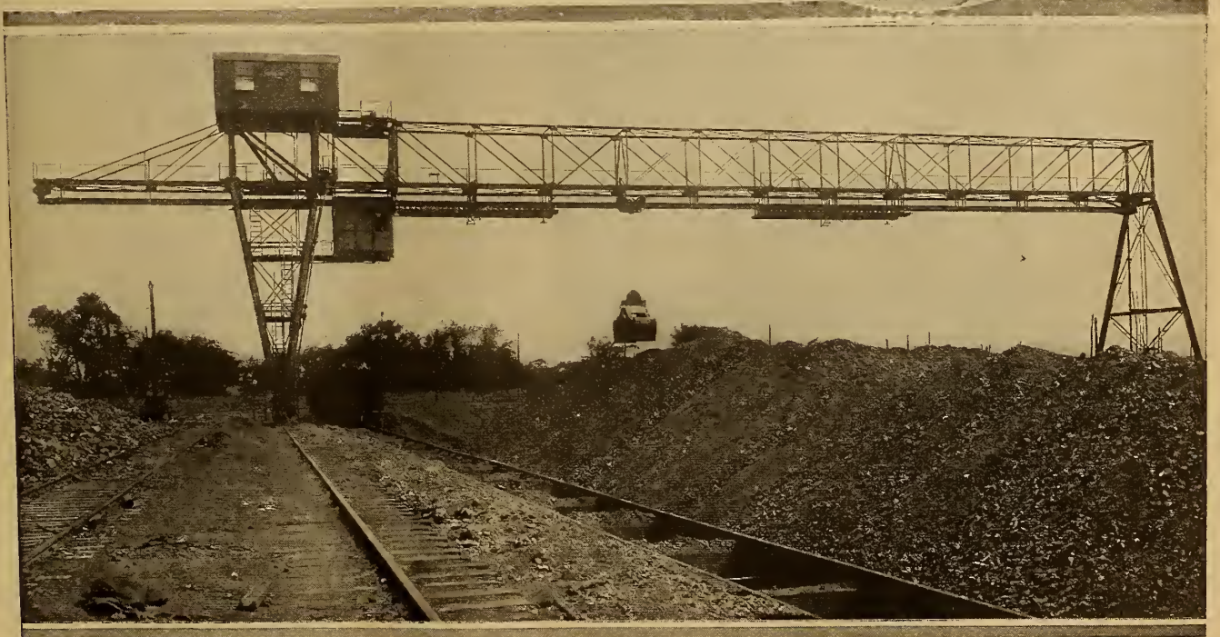
COAL IS NOW HANDLED BY MODERN MACHINERY. BROWNHOIST HANDLING BRIDGE OF THE GENERAL ELECTRIC COMPANY AT SCHENECTADY, N. Y.
