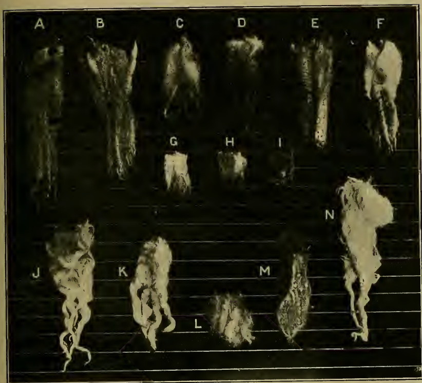
FIG. 1.—Wools and Hairs (the horizontal divisions = 1 inch). A, Lincoln; B, Kent; C, Shropshire; D, Australian Crossbred (46's); E, New Zealand Crossbred (46's); F, Buenos Ayres Crossbred (46's); G, Australian Merino (70's); H, Buenos Ayres Merino (60's); I, Cape Merino (64's); J, Turkey Mohair; K, Cape Mohair; L, Cashmere; M, Camel's Hair; N, White Alpaca. Note. —The presence or absence of grease on these natural wool staples has affected the colour.
