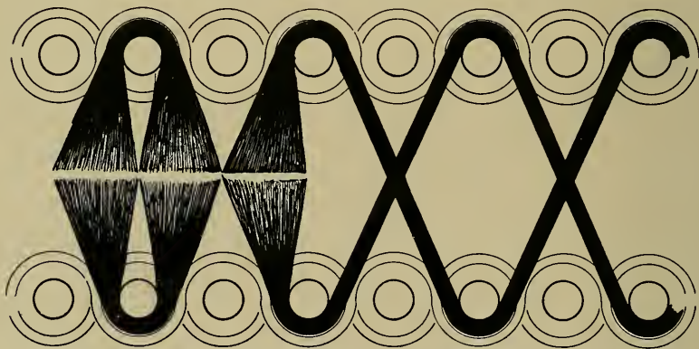
FIG. 45.—Illustrating the Production of Double Plushers, i.e. , Two Single Pile Fabrics, face to face.
