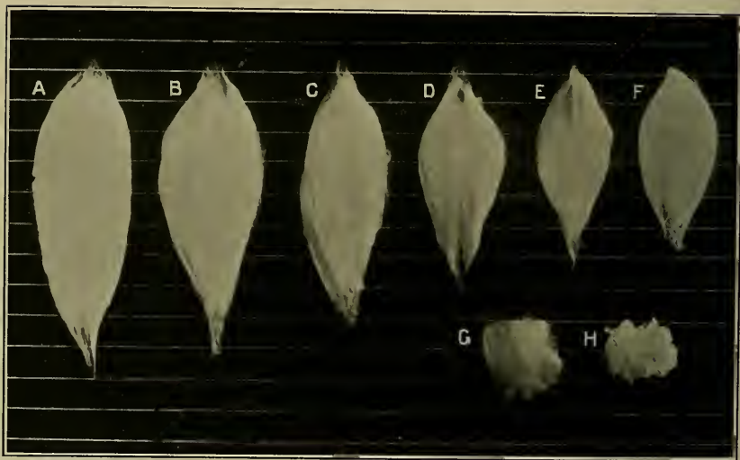
FIG. 22.—Spun Silk Drafts (the horizontal divisions = 1 inch). A, B, C, D, E, and F are 1st, 2nd, 3rd, 4th, 5th, and 6th drafts; G , the shorts, and H the noil.
