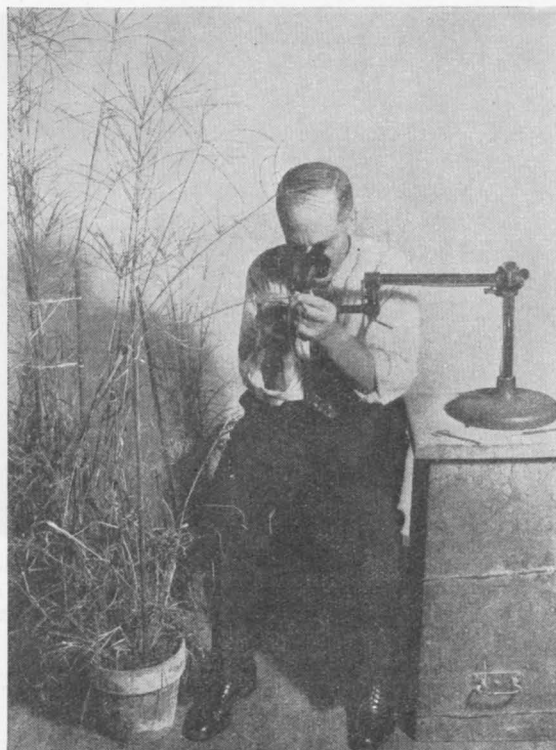
Figure 25.—A binocular microscope with horizontal arm adjustment as used in the emasculatation of woolly fingergrass for cross-pollination in the greenhouse.
