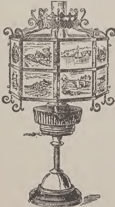
Fig. 32. Lamp-shade for showing off transparencies. Fits the rim of any ordinary duplex lamp, and has grooves to carry the transparencies intended for display. A light touch is sufficient to cause the holder to rotate, so that in turn all the pictures are brought in view.
