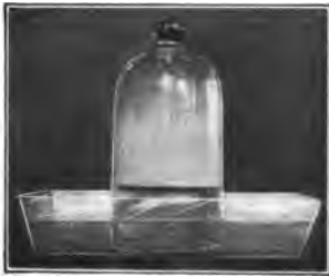
An experiment that shows the air contains about four fifths nitrogen.
