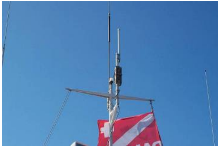
Figure 5. Omni directional antenna on Cypress Sea
