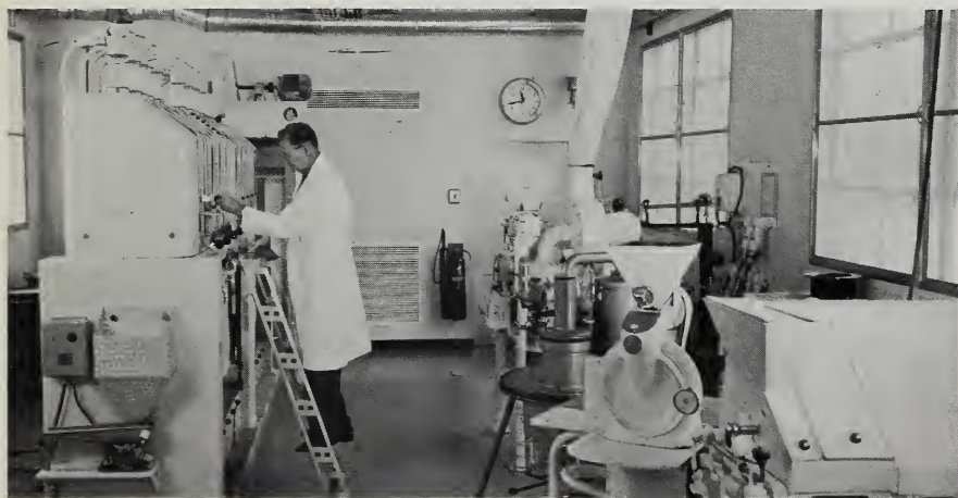
Part of the dry-milling pilot plant where wheat is milled and flour ground finer before separation by air classification into fractions for different uses.
