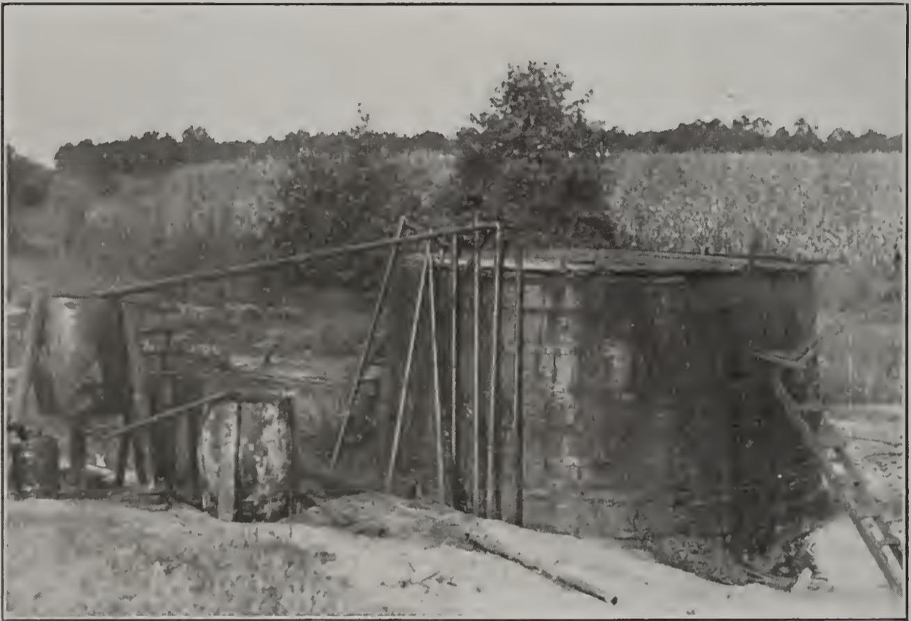
Fig 26. Photograph of the three-barrel siphon gage setup in operation.
