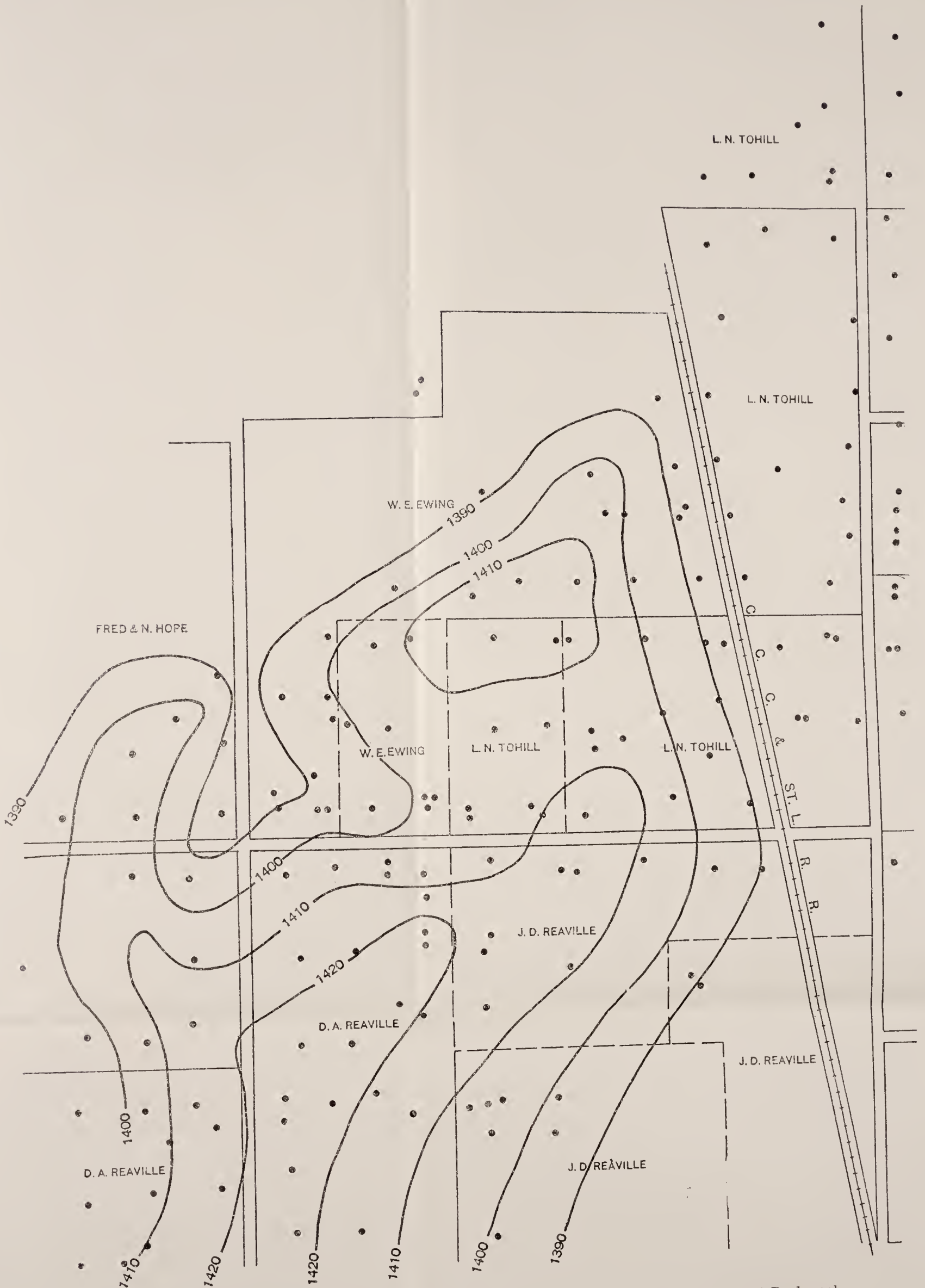
Map showing structure on the surface of the 600 foot "gas sand" in a portion of the Flat Rock pool
