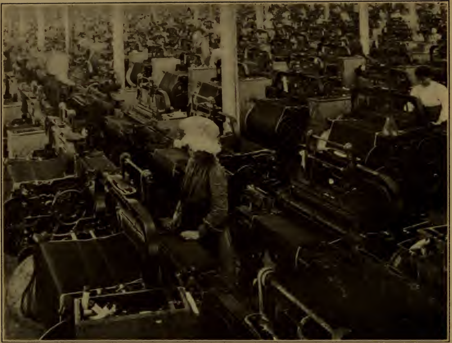
A New England weave room (904 ft. long) 2,000 looms operated by women.
