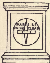
FIG. 26.—Subsidiary Block Indicator.
