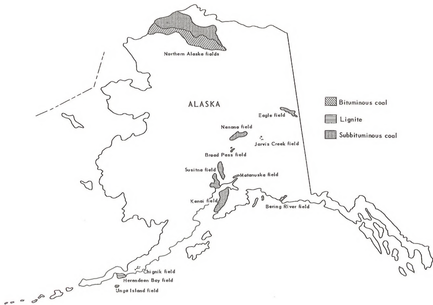
Figure 2-2.--Principal coal fields in Alaska with dominant type of coal in each. (After U.S. Department of the Interior, 1975.)
