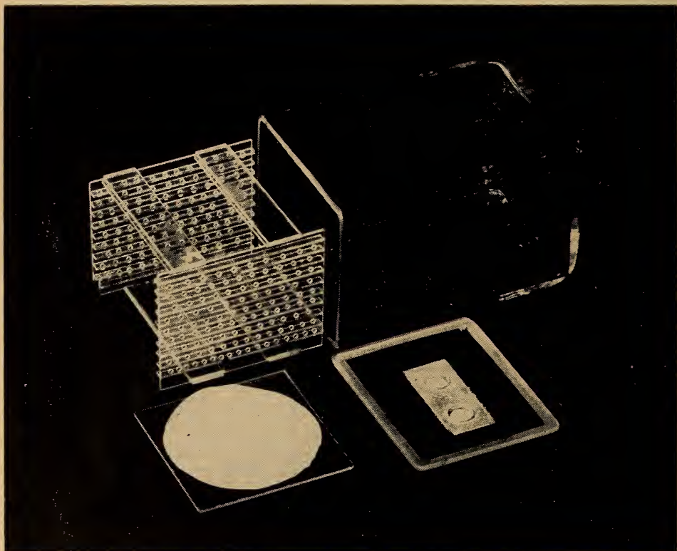
Fig. 3. Museum jar, lid, and rack used in rearing L. tritoma in the laboratory on D. melanogaster .
