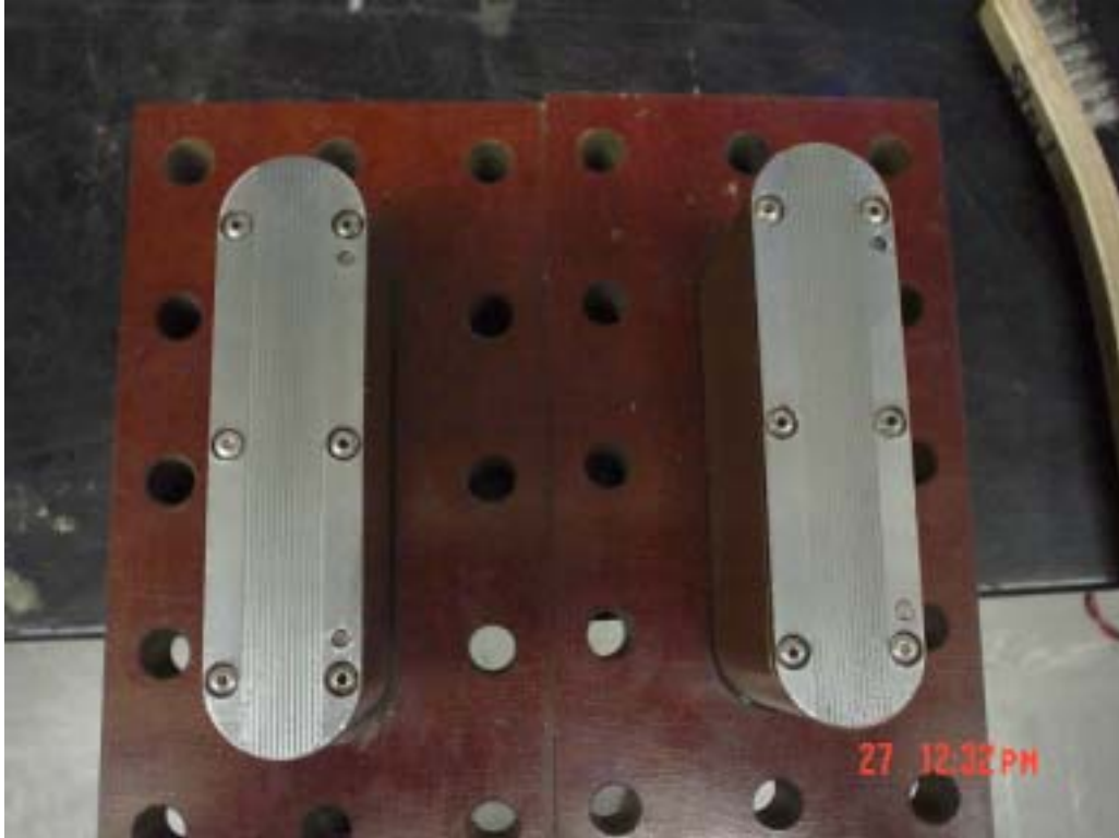
Figure 15. Chrome-plated Copper-Tungsten Rails (Plating done by Barken's Hard Chrome in Compton, California).
