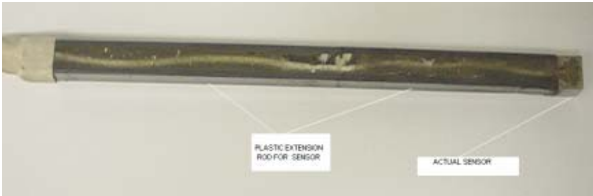
Figure 10. The Sensor Along with its Plastic Extension Rod.
