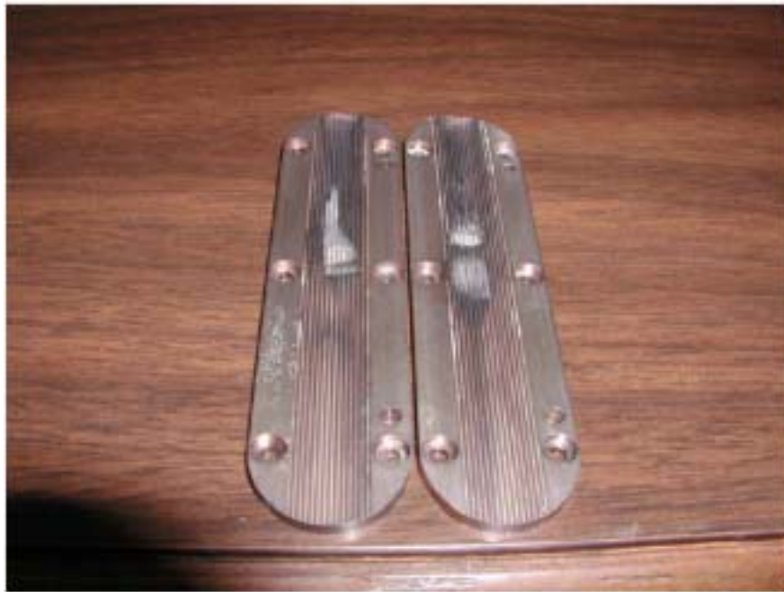
Figure 26. Damage Sustained with No Silver Paste Interface (Conducto-Lube)
