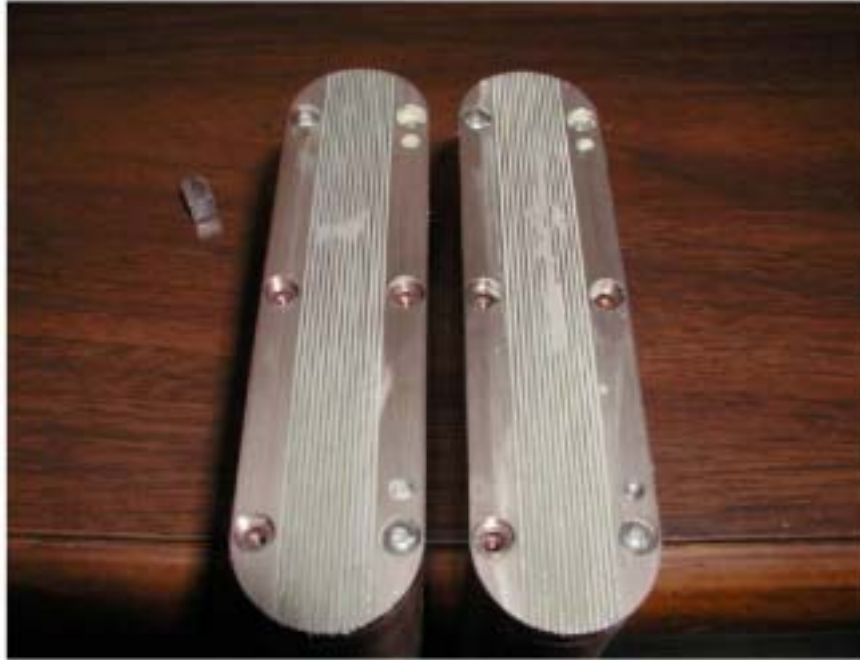
Figure 27. Photograph Taken After a Shot When Paste Was Applied and Low-Voltage Contact Maintained.
