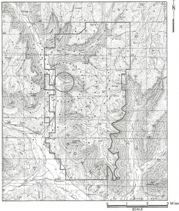
Figure 4.3-1. Receptor locations for Complex I/ISC modeling of sulfur dioxide, nitrogen oxide, and carbon monoxide emissions
