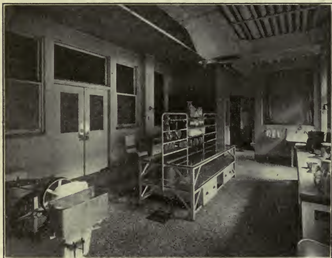
Fig. 18.—A milk station consisting of three rooms. Room 1. For all used bottles, bottle washers, and steam bottle sterilizers. Room 2. A clean room for preparation of formulæ. This room also contains milk separator, fat-testing apparatus and butter churn. Room 3. Pâsteurizing and sterilizing apparatus.
