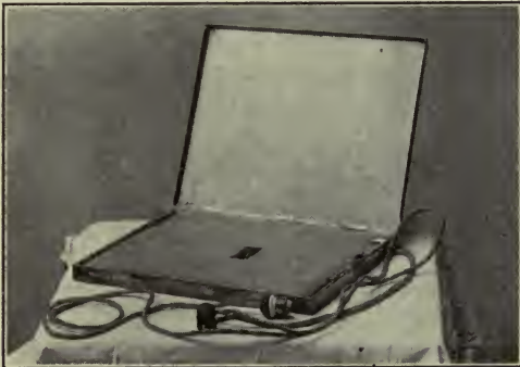
Fig. 20.—An asbestos-lined copper receptacle for electric heating pads for use in the care of premature and debilitated infants ( Hess ). To avoid the danger of fire from short circuits in electric heating pads, a copper receptacle is used, 16 inches long, 13 inches wide, and 1\frac{1}{4} inches high, into which a 12 x 15-inch heating pad is laid. To allow of a maximum radiation from the lid or upper surface of the same, the floor and sides are lined with asbestos sheeting, while the lid is not lined. The cord passes through a small rubber insulator at the side to prevent contact with the metal and injury to the cord. This simple device can be used temporarily in wards and homes where better facilities for the care of this class of infants are lacking. It is to be placed in the bottom of a basket or crib, under the mattress or pillow.
