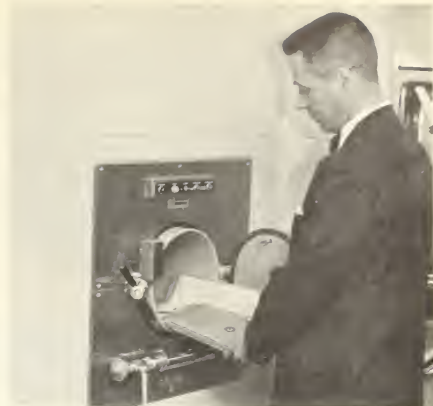
Removing "clean" pamphlets from pass-clave in outside hall after overnight treatment.
