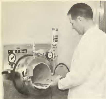
Loading pamphlets into pass-clave inside research unit for sterilization.
