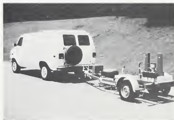
Figure 3—Falling Weight Deflectometer used to assess pavement strength recovery.
