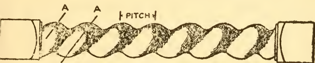
FIG. 79.—SINGLE TWIST TURNING, SHOWING "PITCH."
