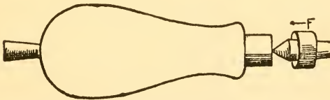
FIG. 27.—TURNING A CHISEL OR FILE HANDLE.
