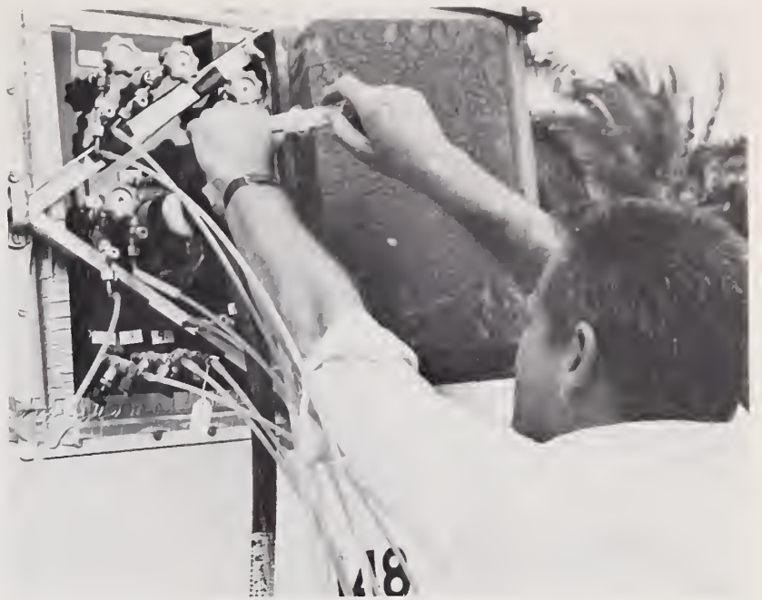
During the fumigation, biological technician William F. Reeder uses a syringe to take a sample of the fumigant from the chamber. A comparative analysis of each sample is made to insure equal distribution of the fumigant within the load (1174X1735-19).
