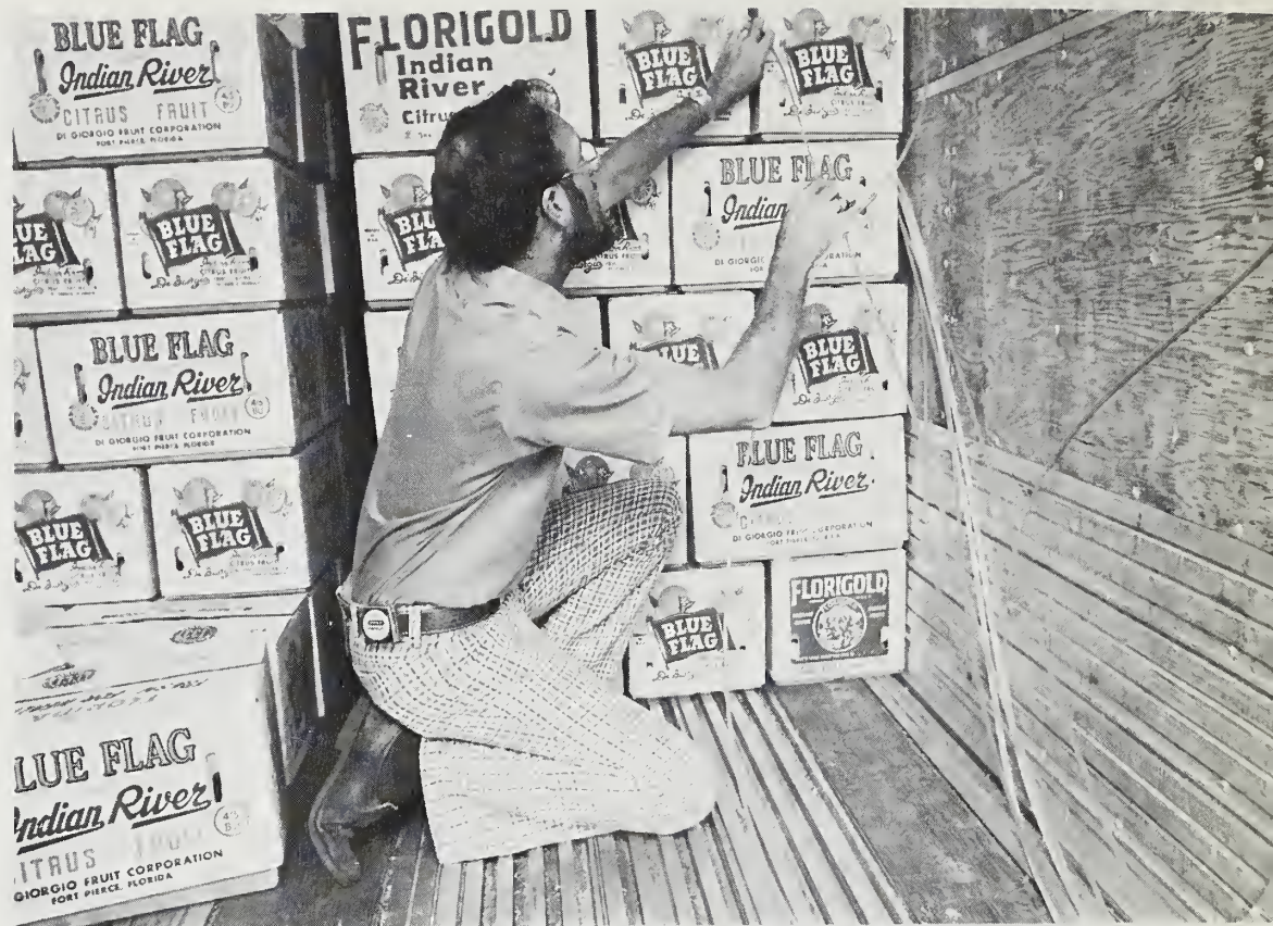
Mr. von Windeguth places plastic tubes between the boxes of grapefruit in the fumigation van to measure gas distribution of the fumigant within the test chamber (1174X1737-5).
