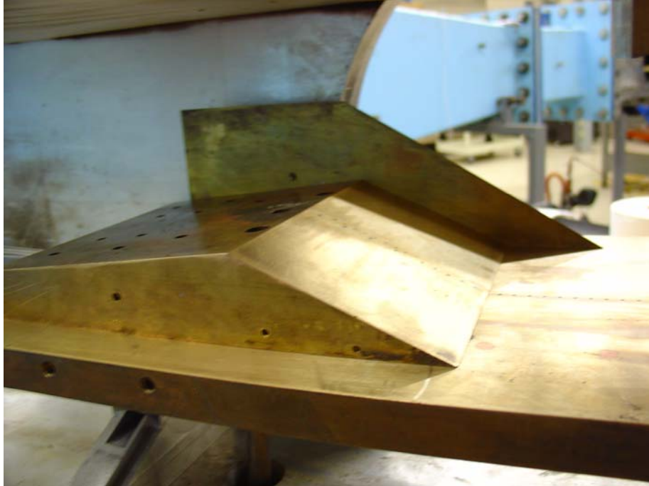
Figure 2.2: 24° compression corner as mounted on flat plate for Mach 2.9 experiments. One aerodynamic fence has been removed to allow optical access for FRS flow visualization.
