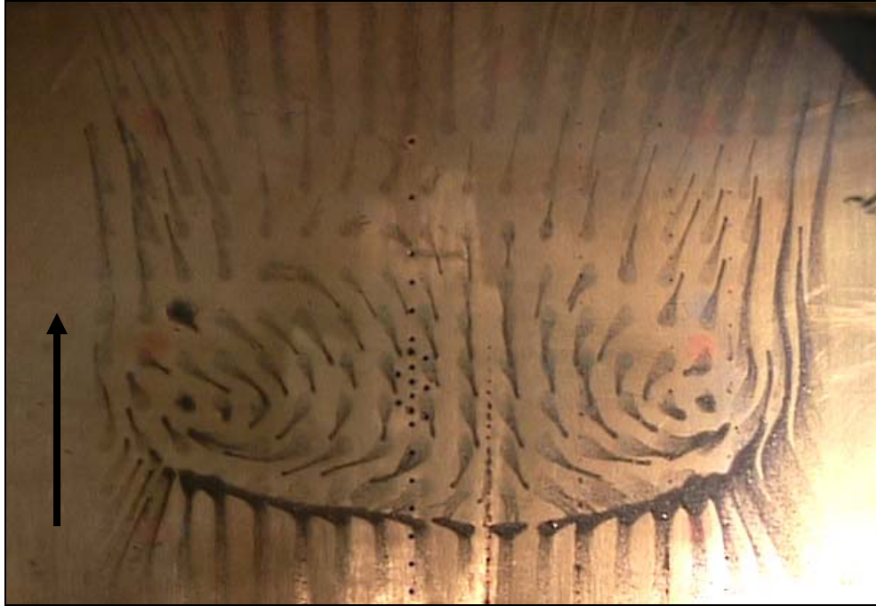
Figure 3.18: Surface flow pattern of the 12° reflected shock interaction at Mach 2.9.
