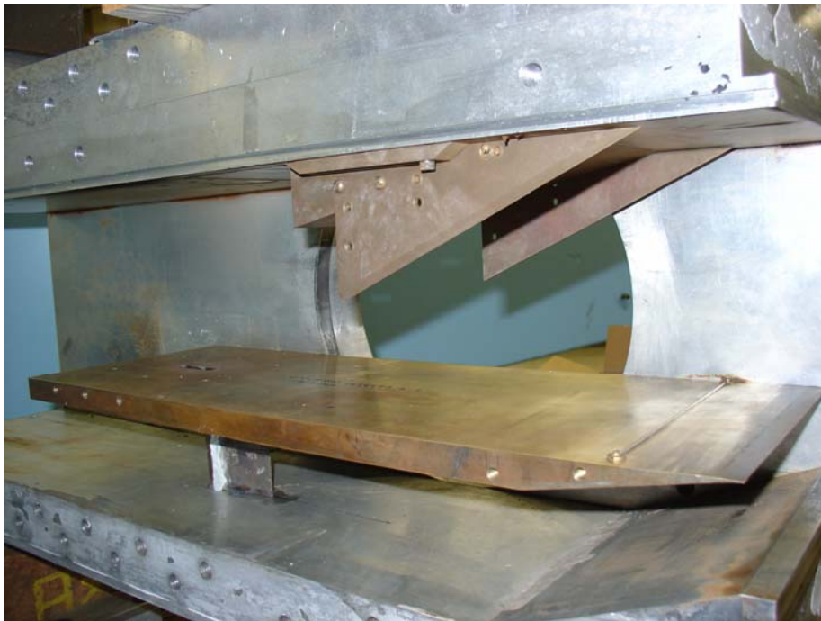
Figure 2.3: 12° reflected shock generator mounted in the ceiling of the test section with aerodynamic fences on both sides of the ramp for experiments at Mach 2.9.
