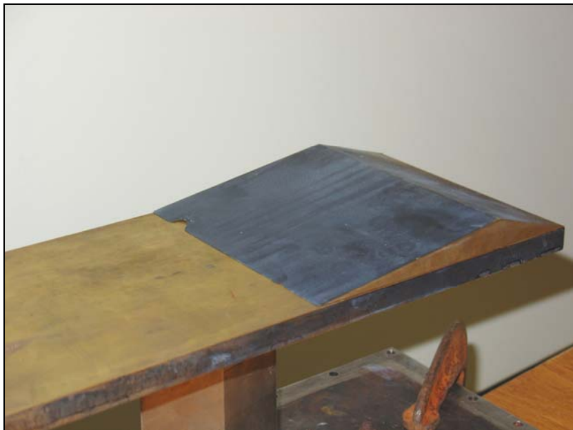
Figure 2.6: 8° compression corner as mounted on the flat plate for experiments at Mach 8. The model was painted black to attenuate background scattering from the laser.
