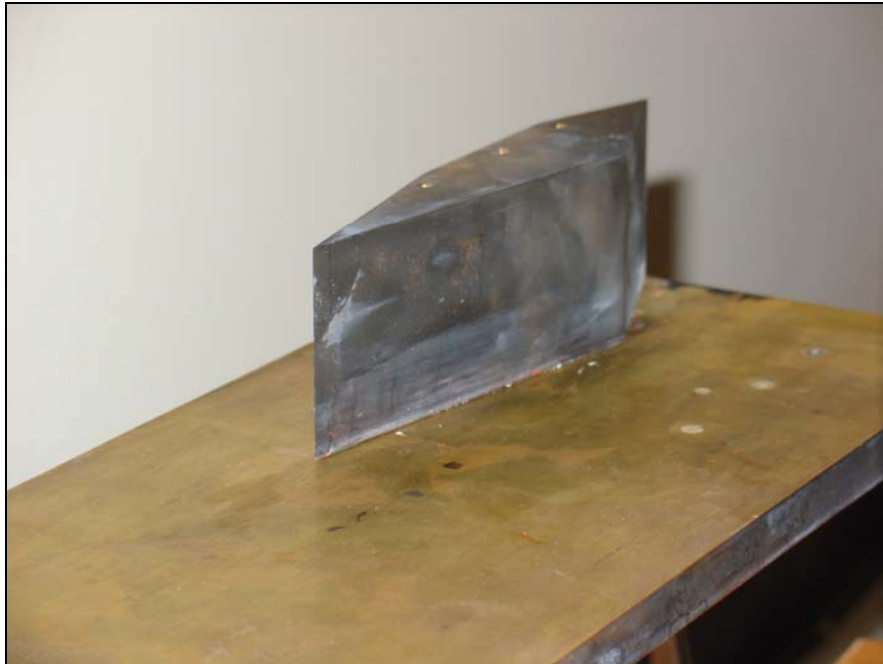
Figure 2.7: 10° sharp fin as mounted on the flat plate for experiments at Mach 8.
