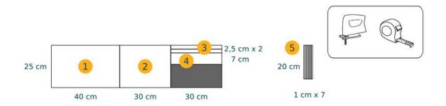
The thickness of the boards making up the box (1, 2, 3 and 4) is 2.5 cm.
