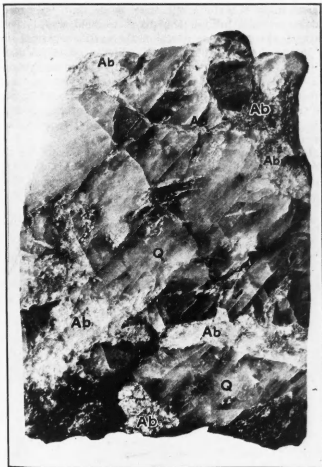
Fig. 7—Quartz partly replaced along cracks by albite, muscovite, and apatite. Peerless dike, Keystone, S. D., 1924, Q, quartz; Ab, Albite
