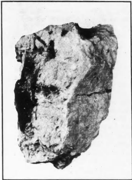
Fig. 16—Thin quartz vein, cutting microcline and giving way to eschynite, which spreads out and replaces the microcline. Petaca, N. M., 1924
