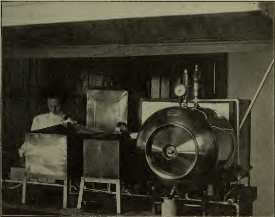
FIG. 5 b . AUTOCLAVE, HORIZONTAL TYPE, CONNECTED WITH STEAM PIPES (All steam apparatus under a hood)
