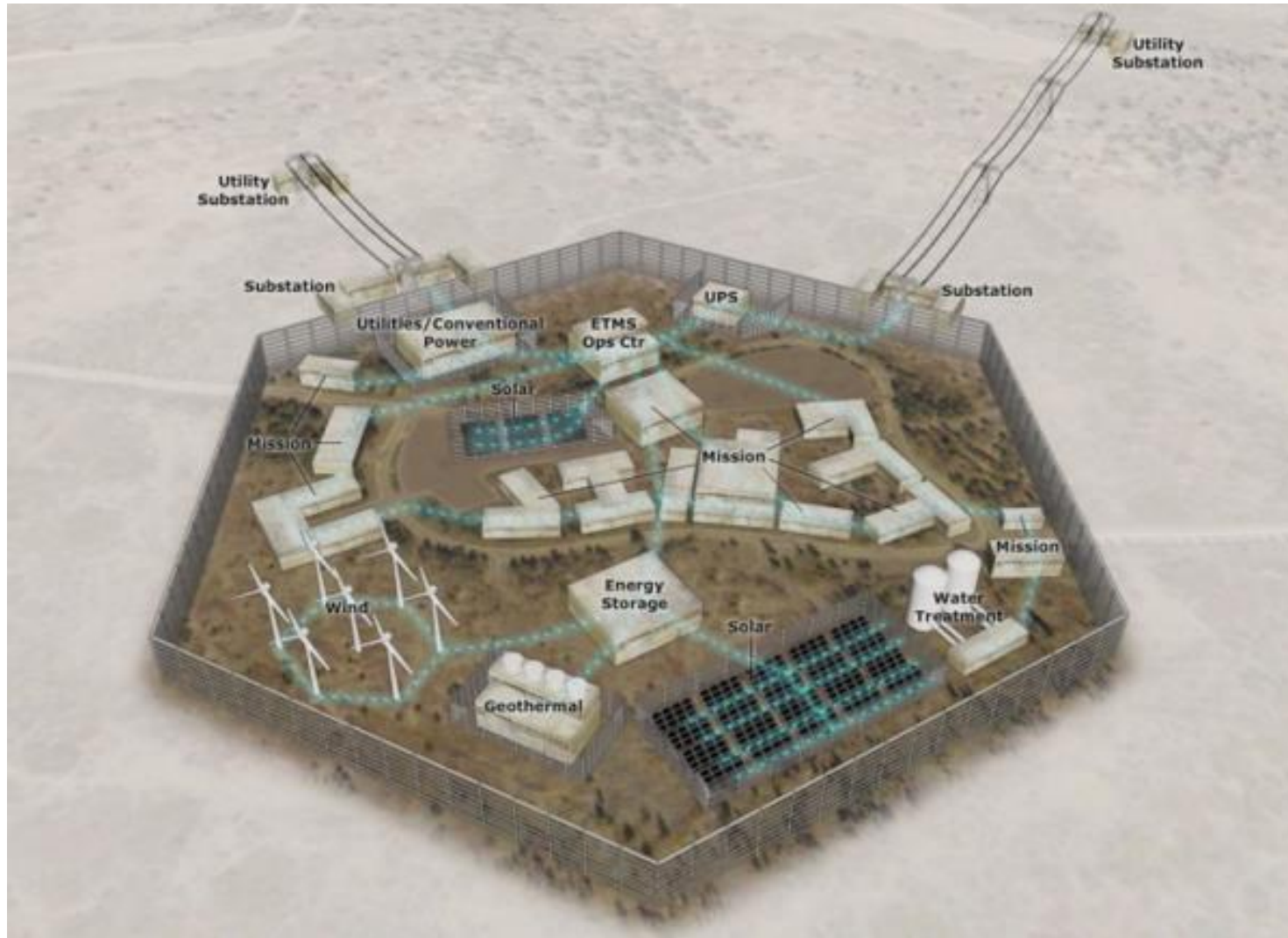
Figure 3. Generic Base Microgrid Implementation. Source: [11].
