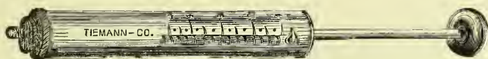
FIG. 63.—BEARD'S PIESMETER.—This instrument consists of a spring in a tube that resists pressure made upon the piston. A scale indicates the amount of pressure upon the spring. It is employed to determine the degree of sensitiveness to pressure in different parts of the body. The forehead, tongue, and cheek are the most sensitive to pressure; the least so are the backs of the thighs and legs.
