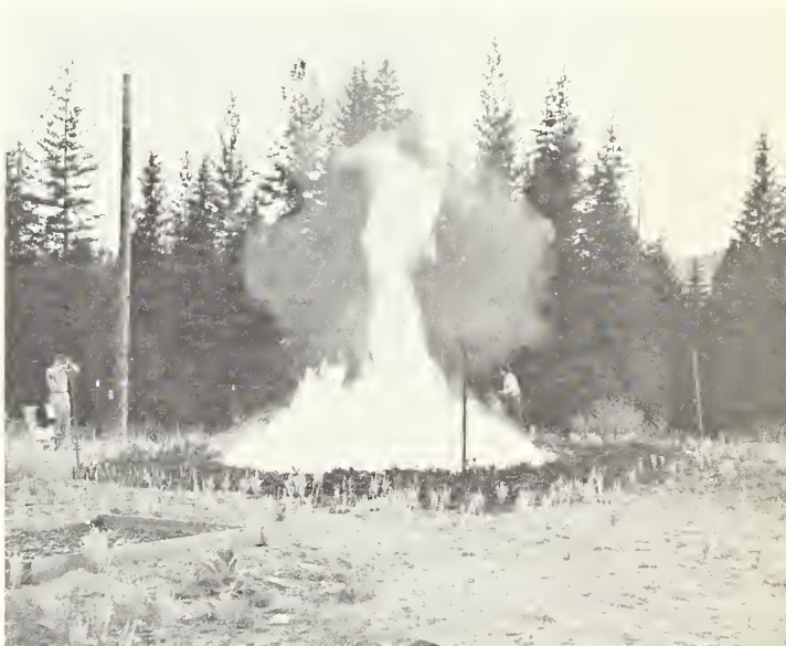
Figure 23. Aging for 1 year only slightly affects peak intensity of fire in slash that retains its needles (western white pine, 32.5 tons per acre). Upper , current year's slash; lower , 1-year-old slash.
