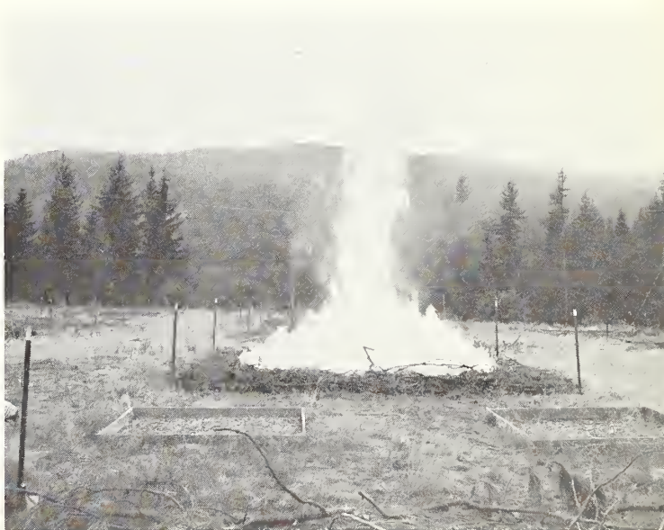
Figure 21. Effect of fuel weight on peak fire intensity in fresh western larch slash: upper, 7.5 tons per acre; lower, 32.5 tons per acre.
