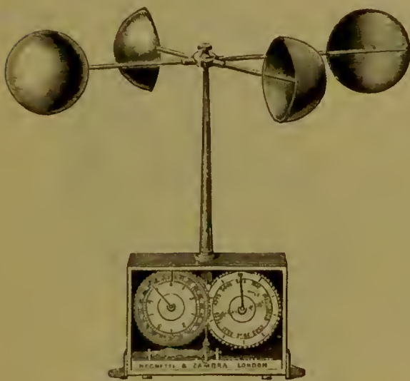
FIG. 59.—Negretti and Zambra's Improved Robinson's Anemometer.
