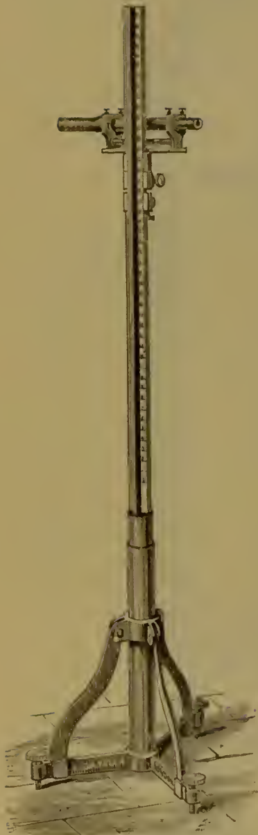
FIG. 35.—Cathetometer, as used at Kew Observatory.
