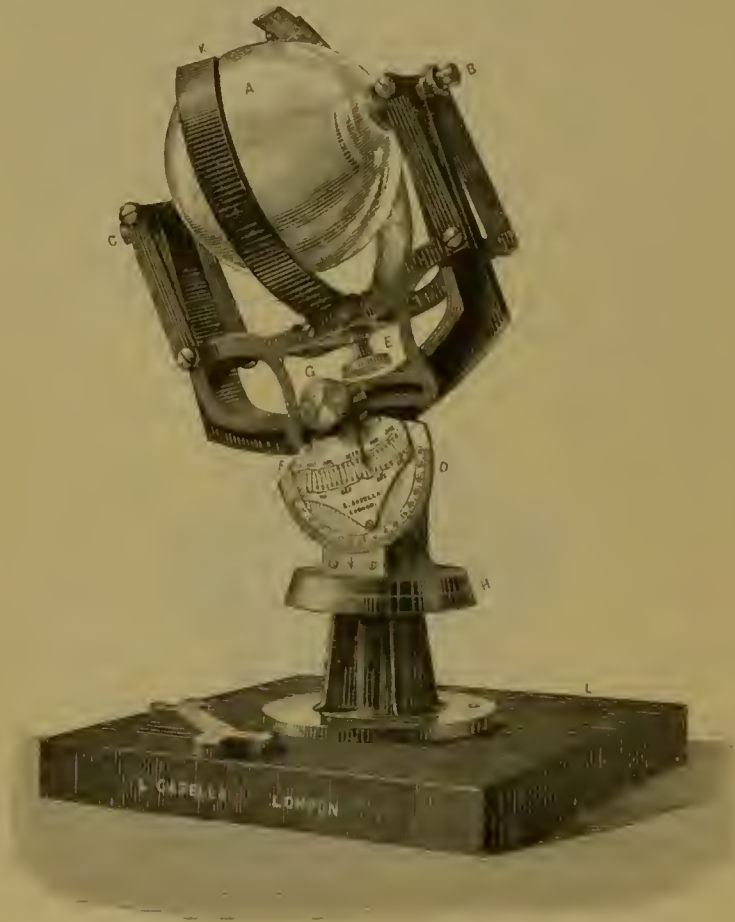
FIG. 14.—The Whipple-Casella Universal Sunshine Recorder
