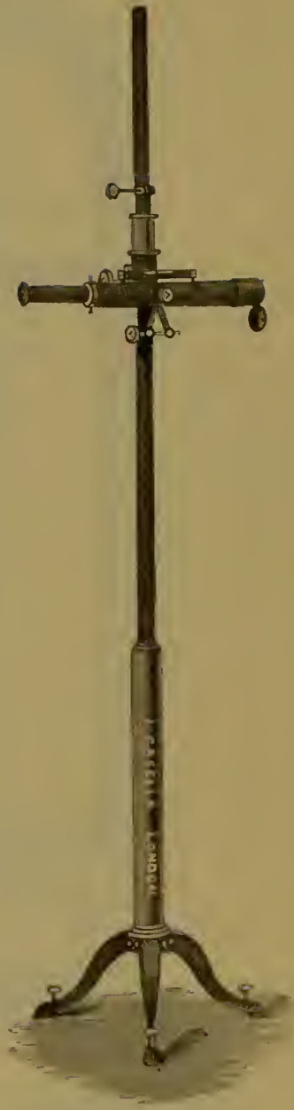
FIG. 36.—Cathetometer, 6\frac{1}{2} feet in height.
