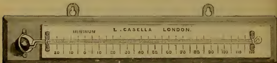
FIG. 3.—Rutherford's Minimum Thermometer, filled with pure alcohol for ordinary registration, engine-divided on the stem.
