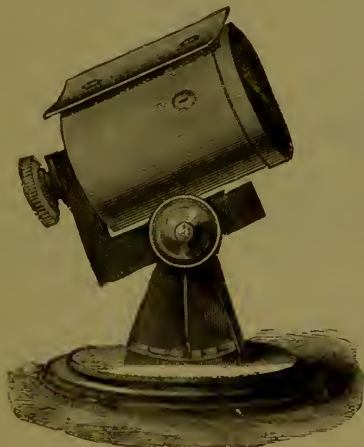
FIG. 15.—Jordan Photographic Sunshine Recorder.
