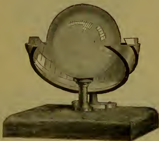
FIG. 13.—The Campbell-Stokes Sunshine Recorder.
