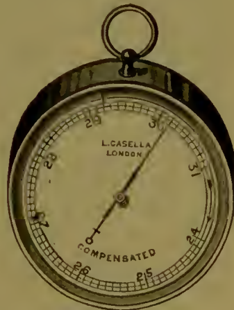
FIG. 28.—Extra-sensitive Aneroid Barometer.
