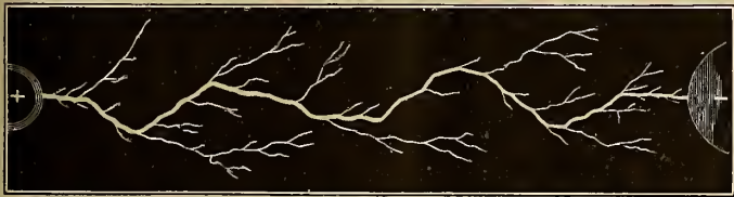
Fig. 22. "Spark" discharge from a static machine.
