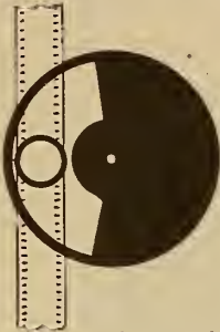
Fig 7—Lens and shutter as set for interiors and faint light—both nearly “wide open”—Lens F/4 Time 1/36 second.
