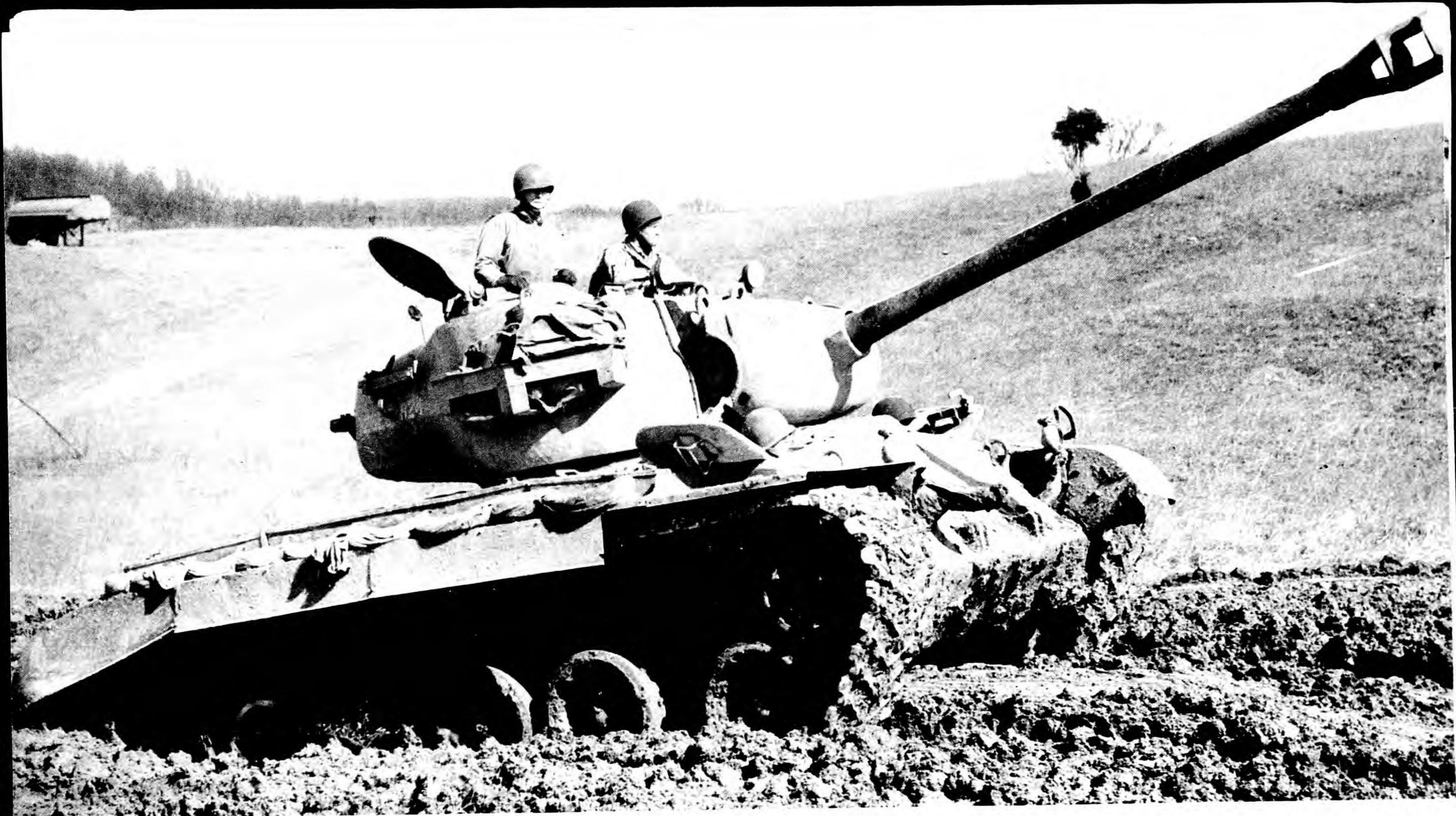
The new M-26 (General Pershing) tank. It is heavier than the Sherman and has a lower silhouette. Increased fire power is provided by the 90-mm. high-velocity gun.
