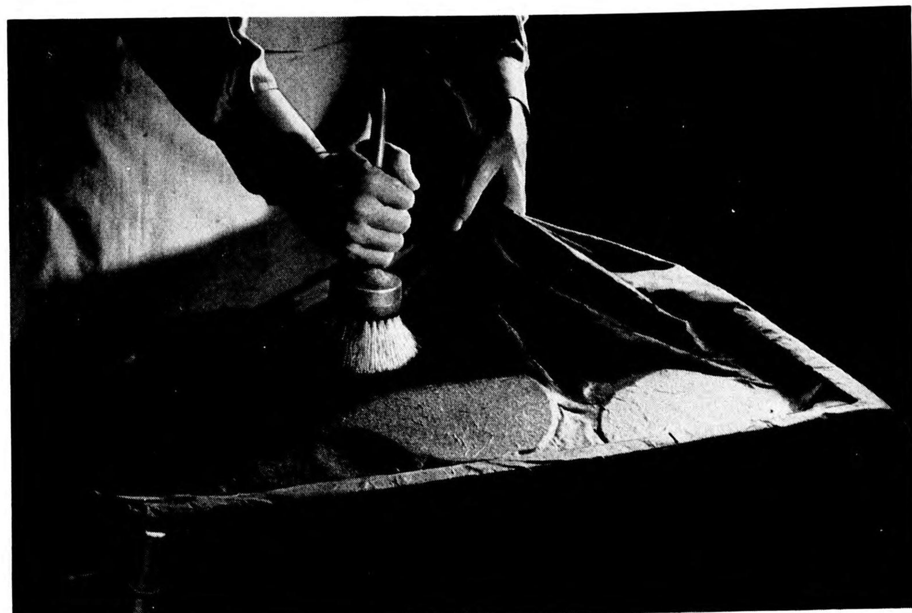
The model-maker soon learns how to stretch molding paper while tamping to prevent wrinkles. See Section 18.
