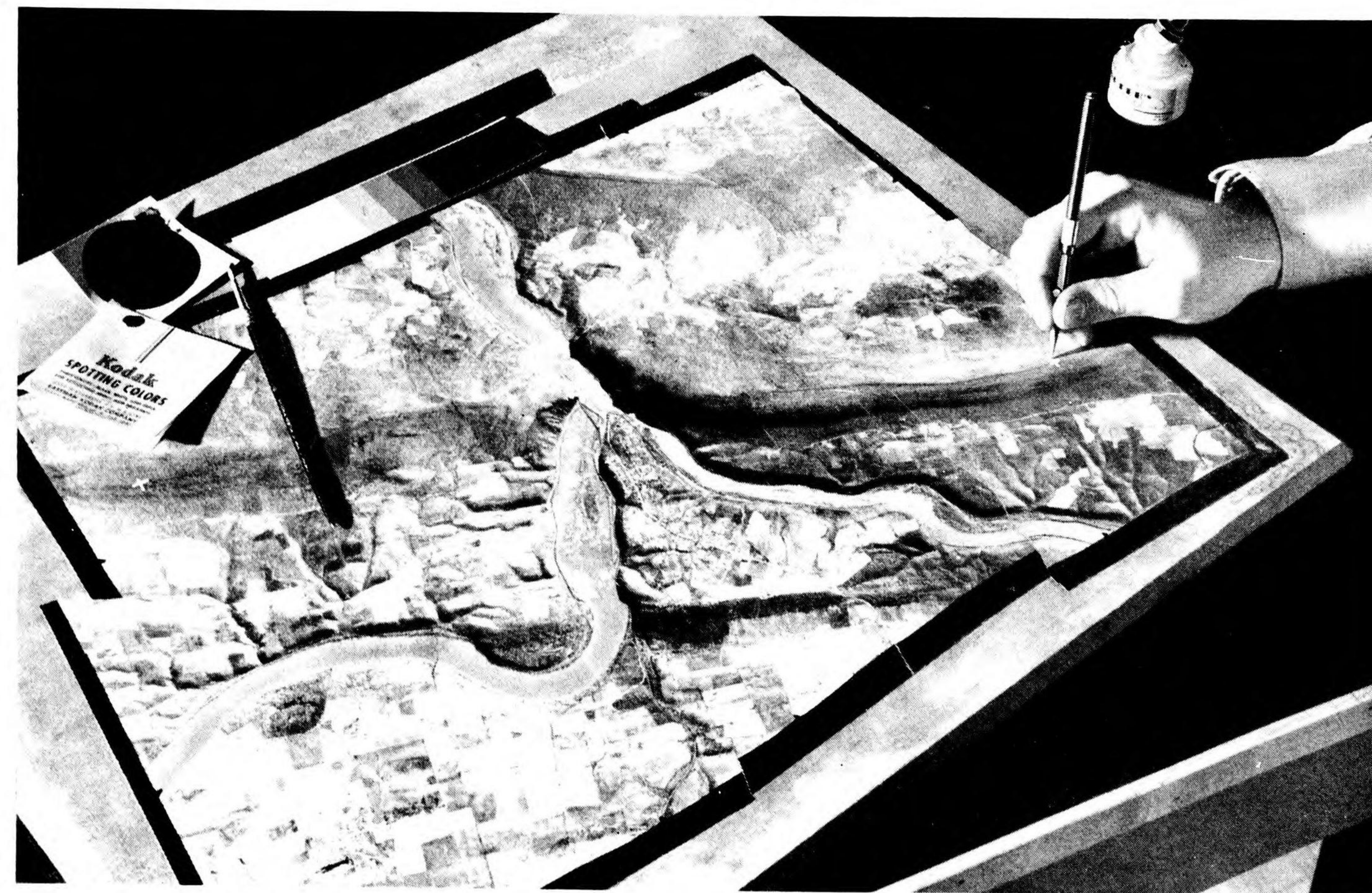
A photo mosaic being prepared as a photo original. Note the white crosses which are added as registration marks. The Gray Scale is attached. Spotting colors have been used.
