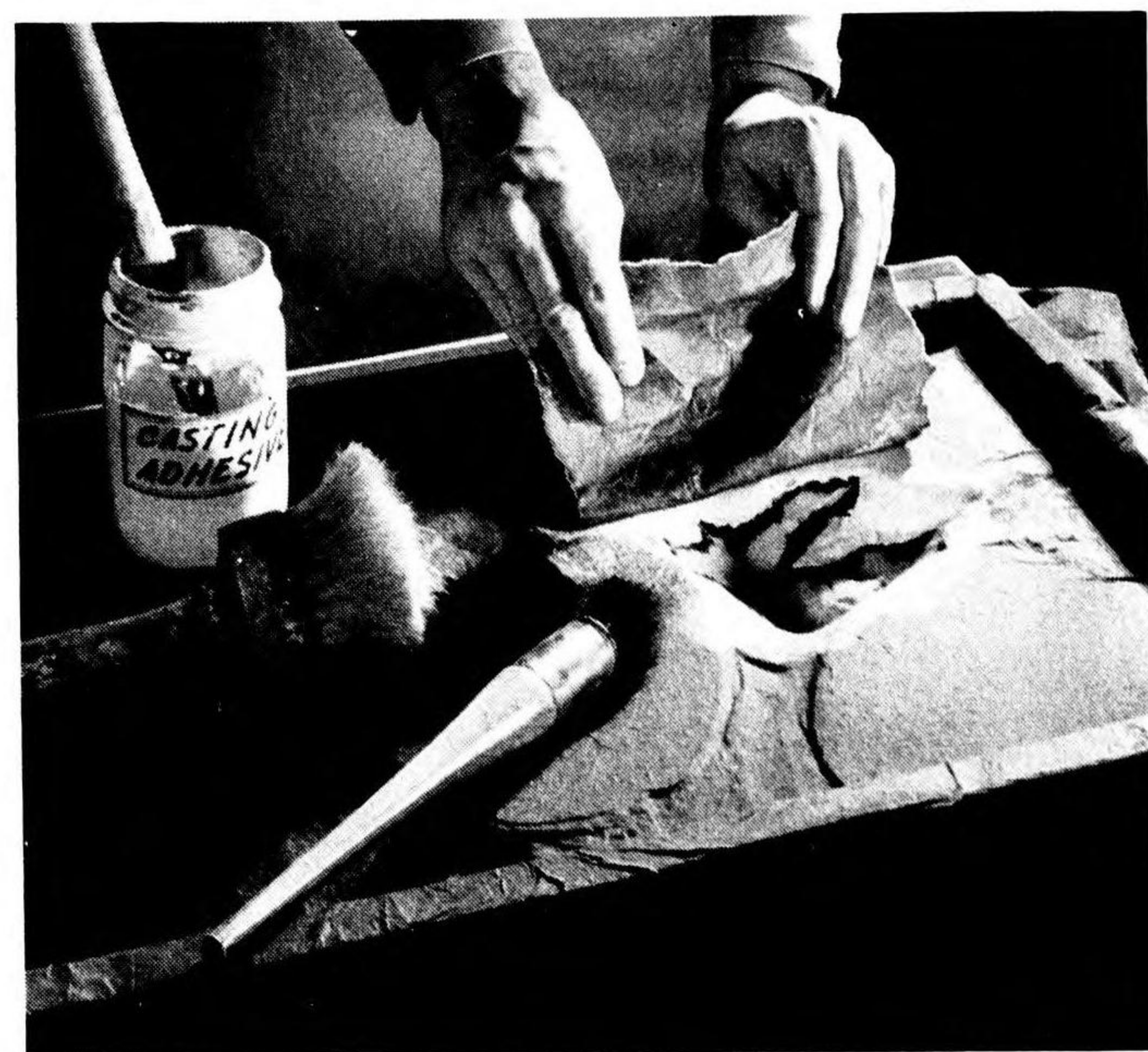
In extra-steep areas, the molding paper is carefully torn, and then patched, as shown here. See 18 (i).
