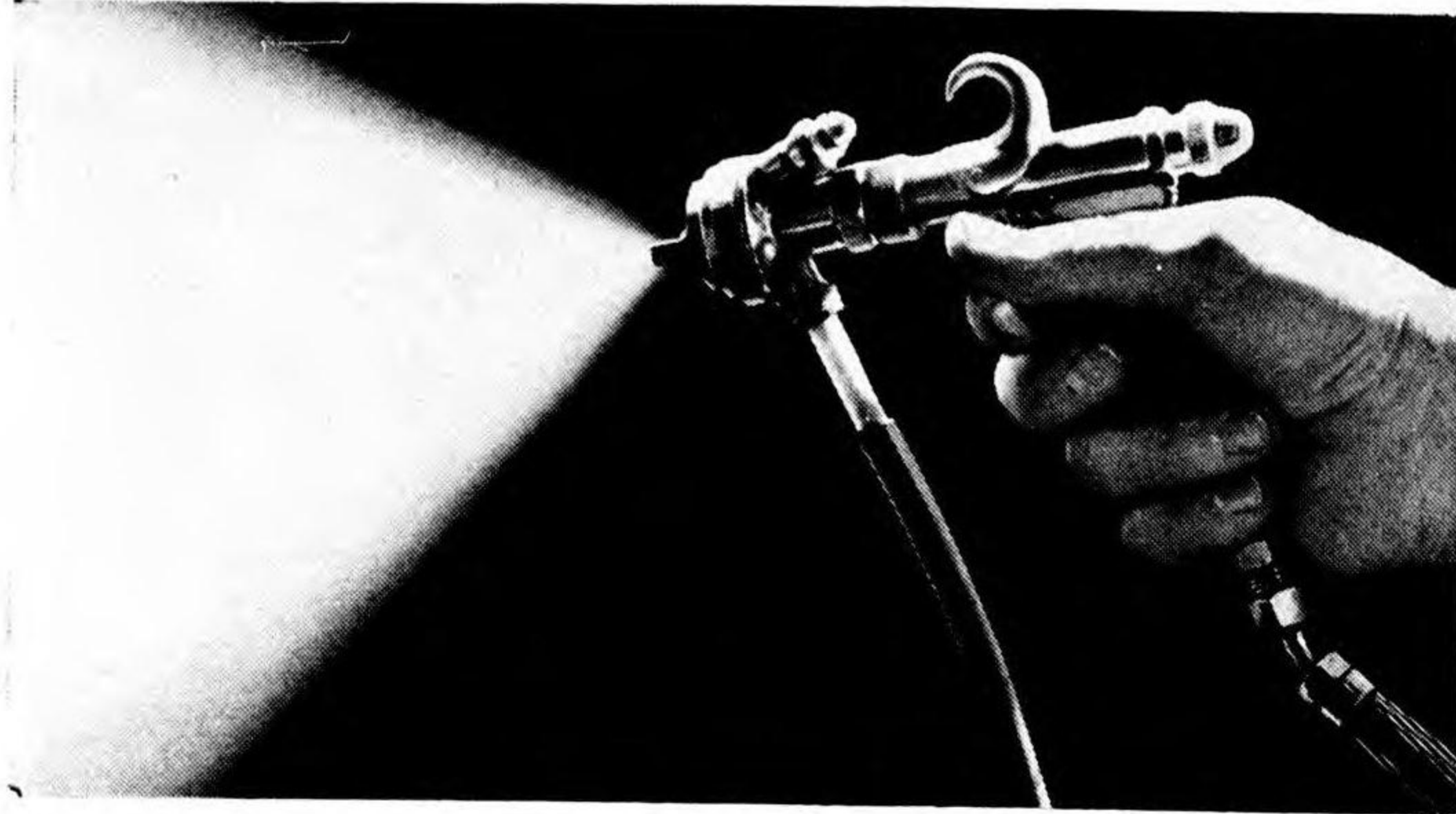
With the fan turned on, the Gun throws a fine flat stream, as though applied with a brush. See 32 (i).
