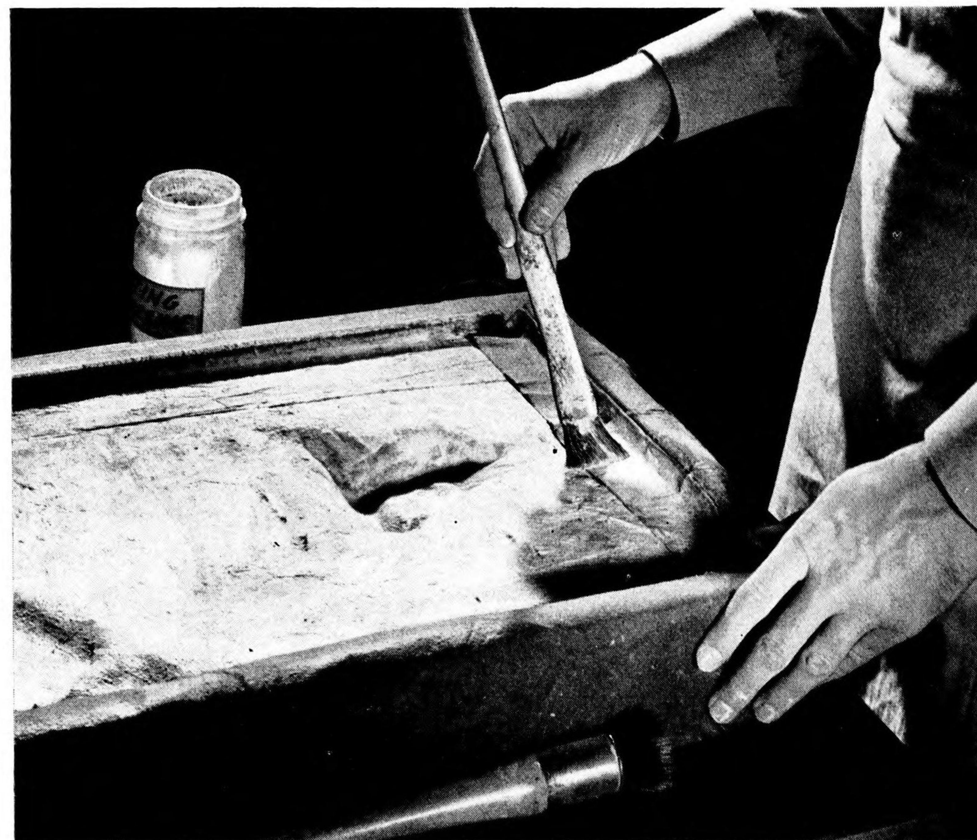
Overlap of the three sheets of paper is folded back to form strong base edges. Casting Adhesive is spread between the sheets of paper. See Section 22.
