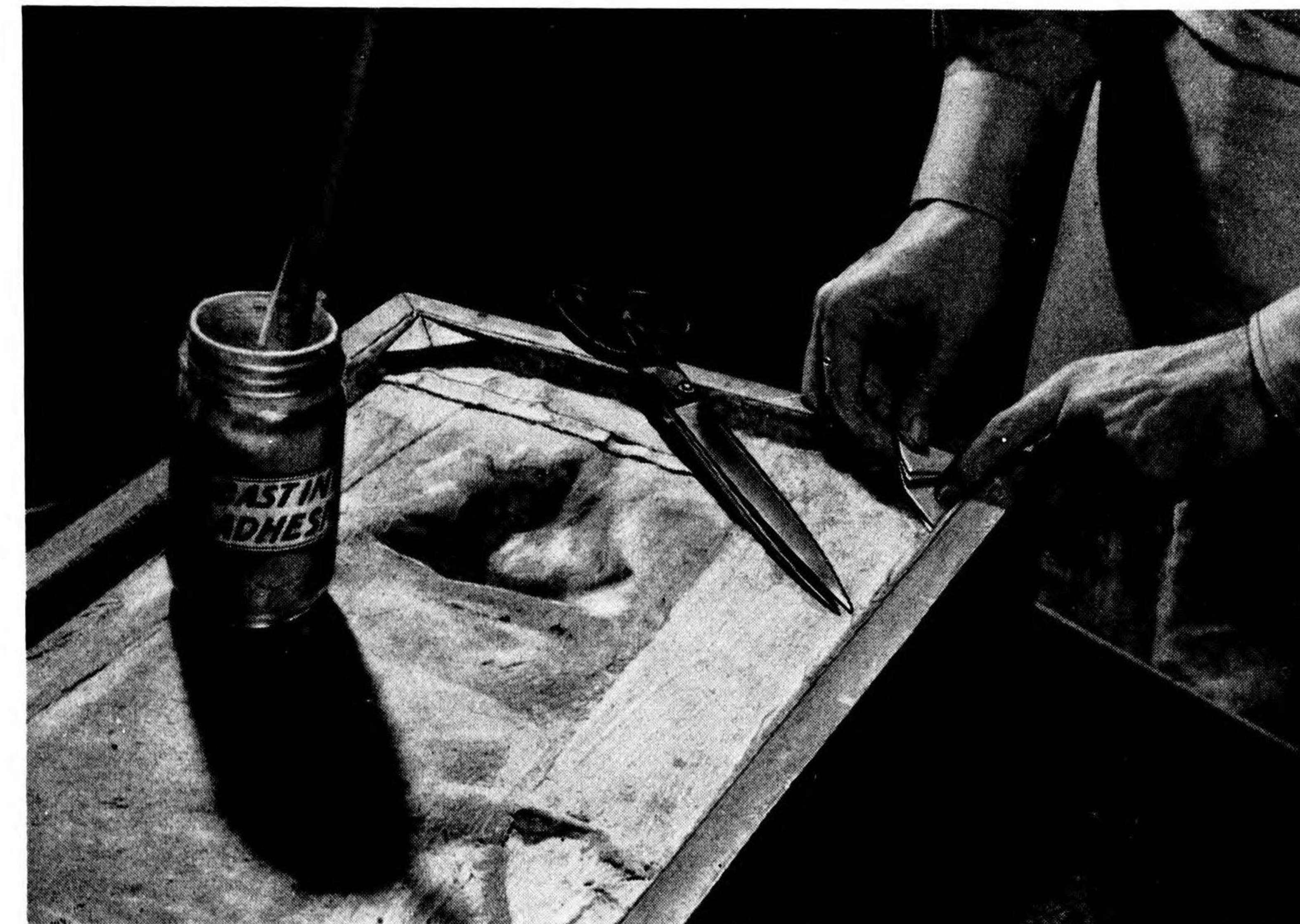
Corners are reinforced with wads of paper, soaked in Casting Adhesive and formed with the fingers. Corners must be strong. See Section 22.
