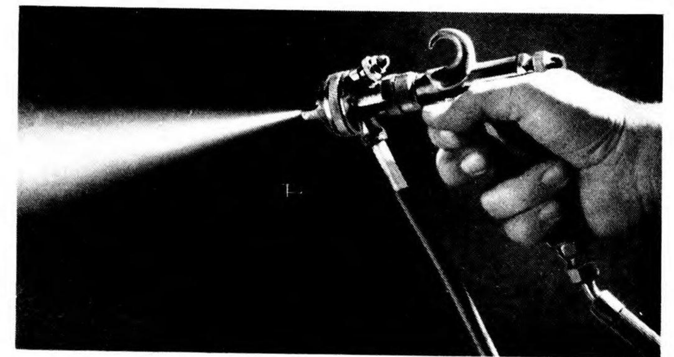
Without the fan turned on, the Emulsion Gun throws a jet-type stream onto the model. See 32 (h).
