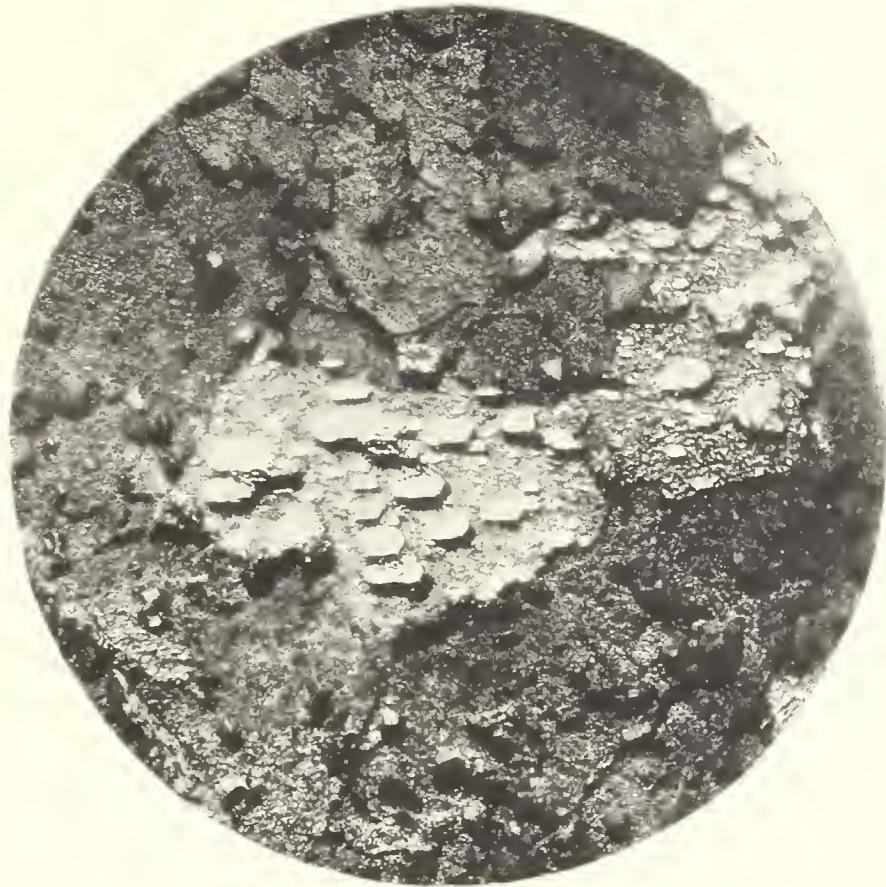
Fig. 5.—Etched sheet-lead. \times 100 .
