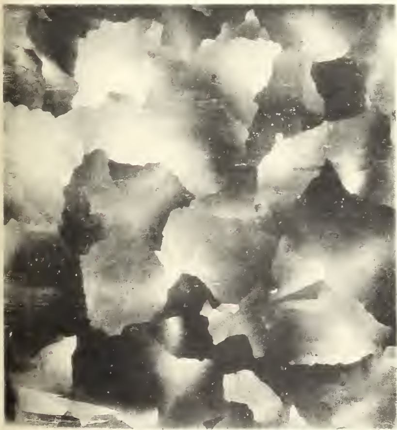
Fig. 28.—Tin-plate, etched. \times \frac{1}{2} .
