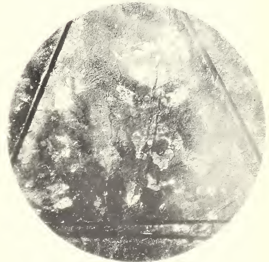
Fig. 15.—Same sheet lead. \times 12 . After 30 minutes at 200^{\circ} C.
