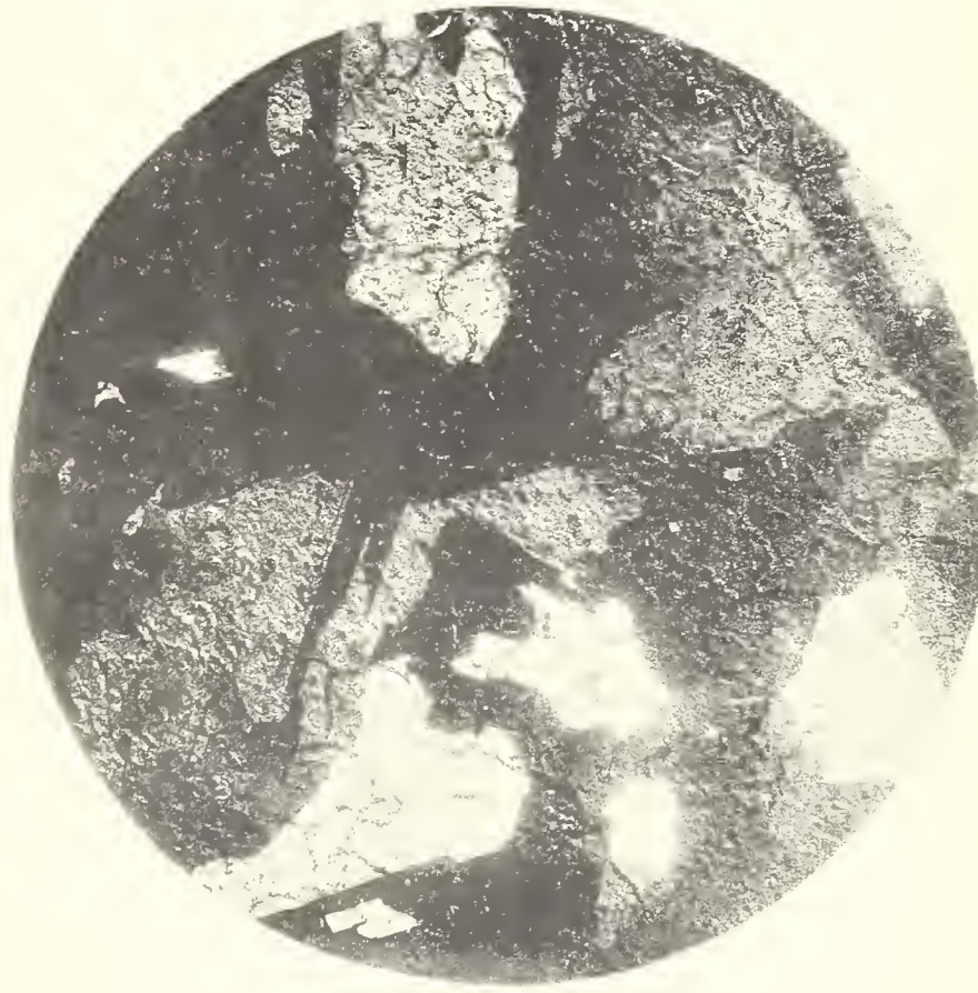
Fig. 19.—Sheet lead. \times 12 . Another part of the same specimen as Fig. 18.
