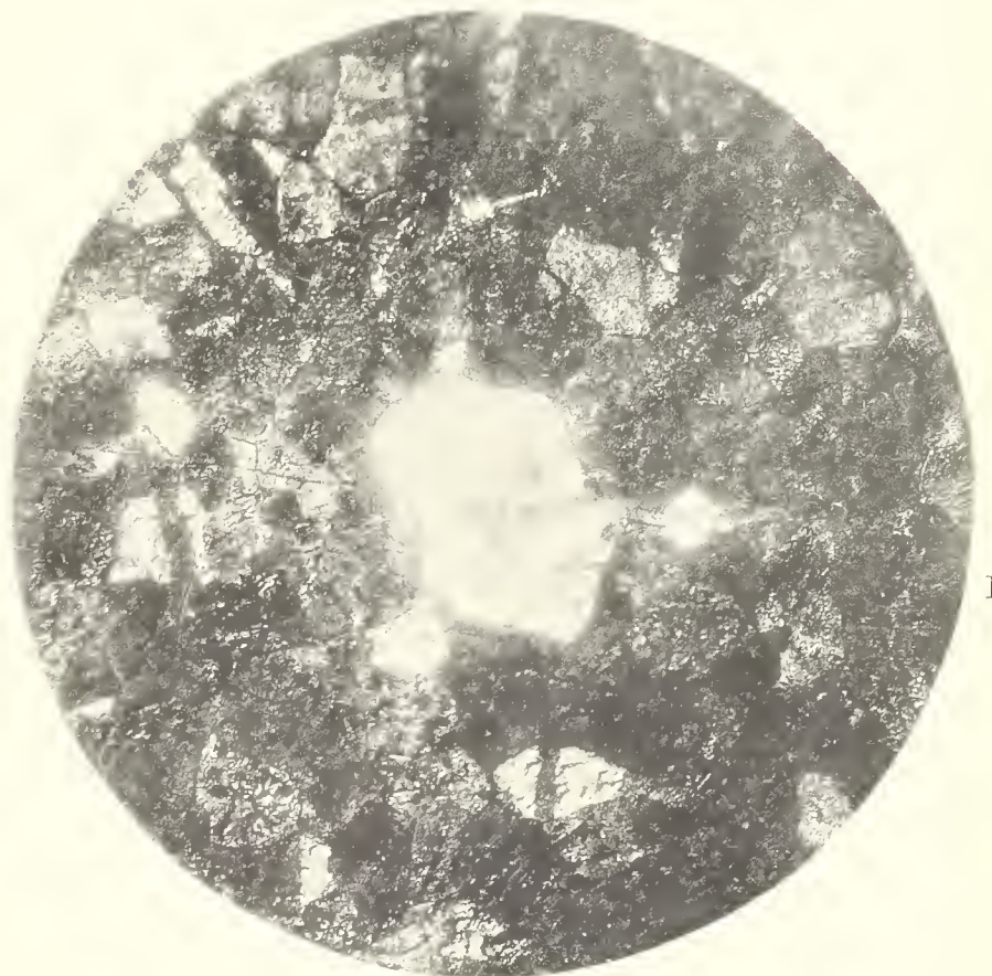
Fig. 38.—Weld in Lead, with eutectic. × 30.
