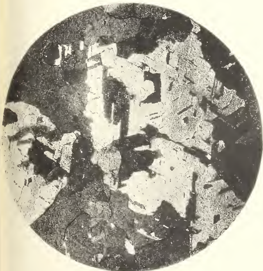
Fig. 3.—Crystals in sheet-lead showing twins, oblique light. \times 40 .
