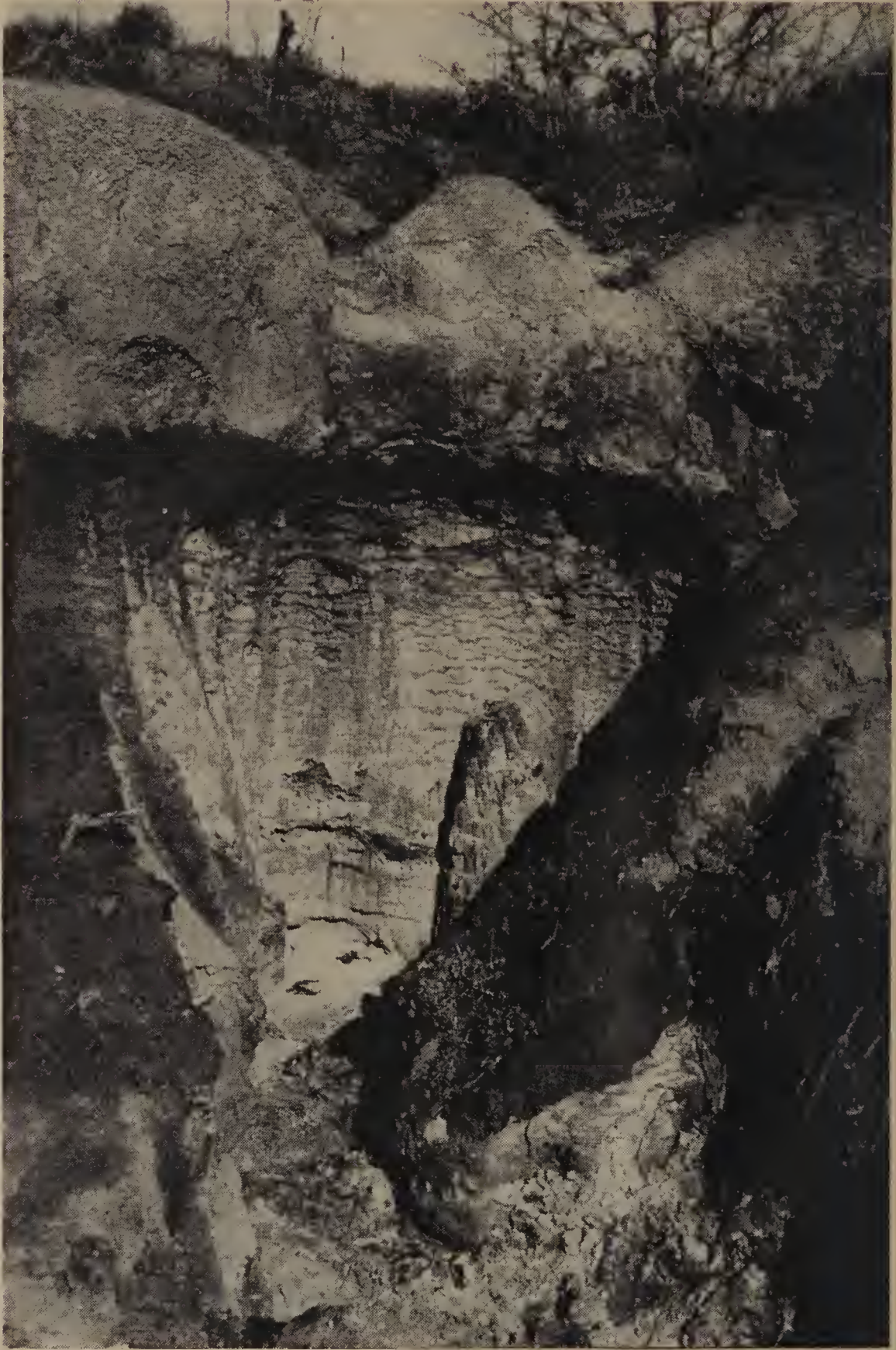
PLATE 2.—Typical Brown Loam profile, showing mantle of loess over Holly Springs sand. Notice undercutting at point of contact
