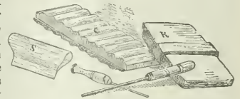
FIG. 10.—Currying Apparatus. C, pommel; R, raising board; S, slicker.
