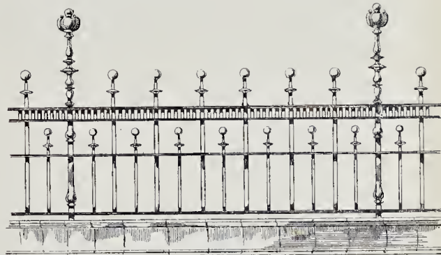
Iron Railing along Cornice, Strand and Savoy Court Elevations.
