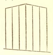
The two upper sloping lines represent two drains on the higher level which intercept the water draining from the hill, and the parallel lines running down the descent through the garden, indicate drains either discharging into a pond or brook, or connecting with a main drain which conveys the water to some proper outlet of discharge. If the land is on a ridge the lateral drains should be right up
