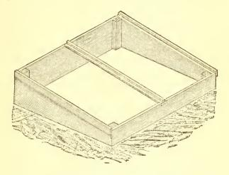
The box or frame should be two feet high at the back, and sixteen inches at the front, and should be made of inch and a half plank. When two or more sashes are used, brace-pieces six inches wide must be set across the frame, from back to front, and dovetailed into each, so as to carry the sashes and stiffen the frame. On these braces a parting-strip must be nailed, in order to separate the sashes and cause them to run true. On each side or end
