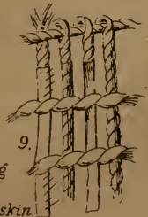
Diagram of the Structure of Mat with Feathers woven in.
