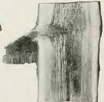
FIG. 4.—THE FRUITING BODY OF A WOOD-DESTROYING FUNGUS GROWING ON A LIVING FIR, SECTIONED TO SHOW HOW THE FUNGUS HAS DESTROYED THE WOOD AND HAS THEN GROWN OUT THROUGH A BRANCH.
