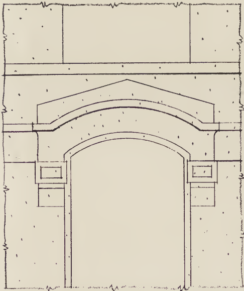
FIG. 10. DESIGN FOR DOORWAY TREATMENT IN CONCRETE.
