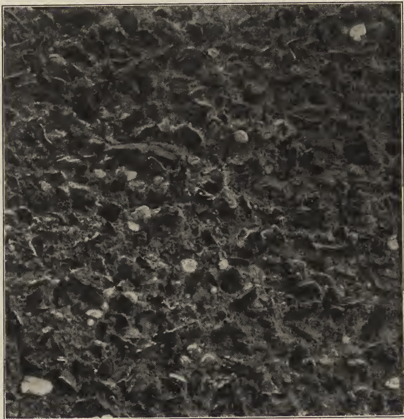
FIG. 6. SHOWING CONCRETE SURFACE ETCHED WITH SOLUTION OF HYDROCHLORIC ACID AND WATER.
