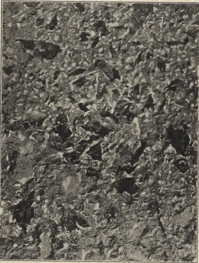
FIG. 9. SURFACE FINISHED BY HAND HAMMER OR AXE.
