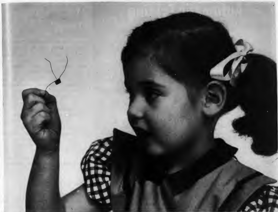
THAT'S A TRANSISTOR, invented at Bell Telephone Laboratories. This tiny electronic device can do many things that vacuum tubes can do and more besides. Though little larger than a coffee bean, it can amplify electric signals 100,000 times.
