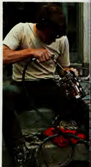
Compressed air and chemicals were used to dry sodden electronic components.
