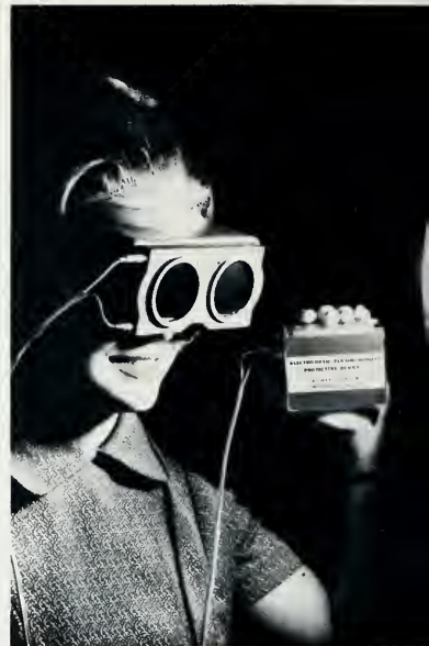
Electro-optic ceramic material in these goggles protects eyes from the brilliant light of the flash. Laminar air flow technology, another Sandia development, was first used here at the operating suite, Bataan Memorial Hospital in Albuquerque. Engineers examine part of an earth-penetrating jeticle used to measure Arctic ice.
