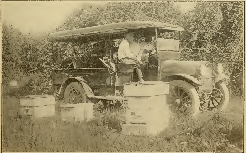
The platform with extractor, engine, tank, wheelbarrow, and the whole outfit, in fact, loaded on the truck.
