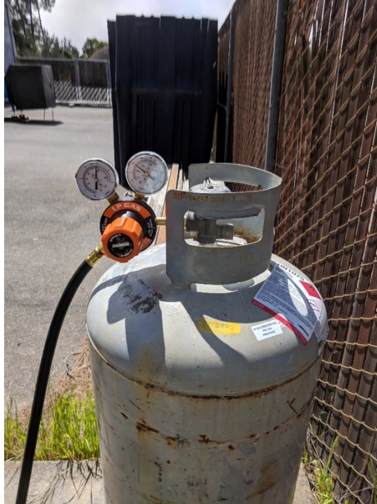
Figure 15. C_3H_8 tank, regulator, and flexible tubing assembly
