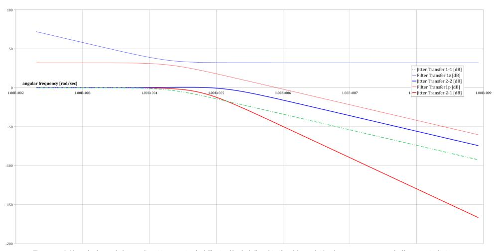
These curves holds good as long as the loop non-linearities are not involved. The signal levels shall not (significantly) exceed either the comparator range nor the filter saturation limits.
